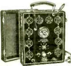
The greatest tube tester value ever offered. Tests all the new tubes as well as the old ones without adapters. Equipped with 4, 5, 6 and 7 prong sockets. Encased in handsome leatherette case with deluxe handle and removable hinge cover. Operates from AC socket. Size 11 x 9 x 5 inches.
