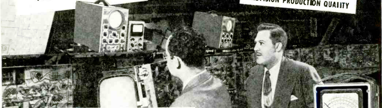
Tele-King Production Test Foreman James Adler and Harry R. Ashley, President of EICO, inspecting the use of the EICO Model 425 Oscilloscope and Model 221 Vacuum Tube Voltmeter at one of the important constant-duty alignment positions on the Tele-King television production line, New York City.
