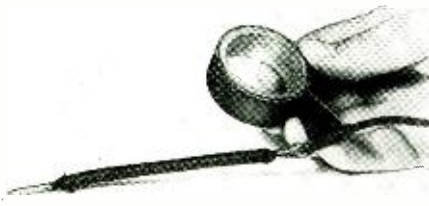
Photo A—Use a 6-inch length of No. 4 rubber covered wire to make a very simple test prod. Remove the insulation from both ends and grind one end to a point. Solder a piece of flexible wire to the other end and cover the joint with tape.
