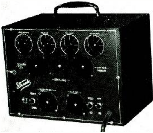
Front view. Tube sockets act as jacks for speaker and cutter.
