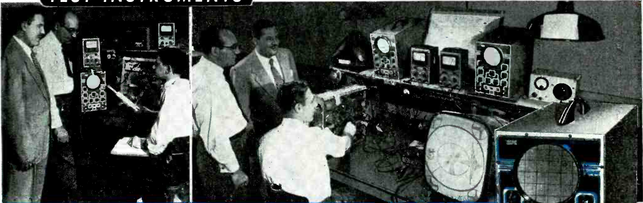
Frank J. Dieli, Majestic's Chief Engineer, and Harry R. Ashley, President of EICO, inspecting the use of the EICO Model 425 5" Push-Pull Oscilloscope, Model 221 Vacuum Tube Voltmeter and Model MVP-1 High Voltage Probe at the important Final Test Position on the Majestic Television production lines.
