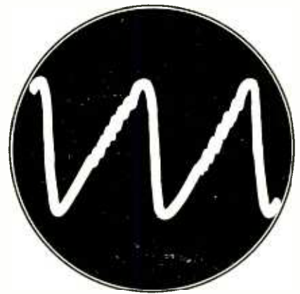
Fig. 5—This waveform was on the grid of the horizontal output tube of a Hoffman 196. Note the excessive ringing.
