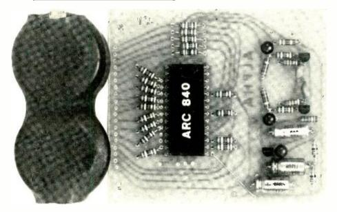
CALCULATOR'S PC BOARD and Its associated parts are seen when keyboard and display are removed. Round objects at left are the re-chargeable batteries wrapped in heat-shrink plastic tubing.
