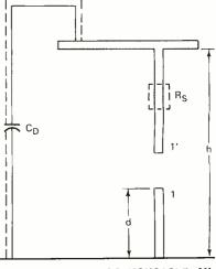
FIG. 2-IMPEDANCE OF MONOPOLE AN-TENNA is measured between points 1 and 1'.
