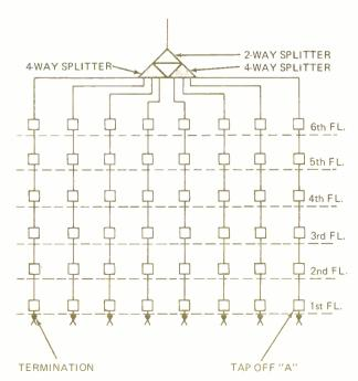
FIG. 4-HOW CABLES ARE LAID OUT in a typical building of moderate height. Three splitters drive the eight feeder lines.
