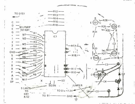
WHERE PARTS ARE MOUNTED on the PC board and how leads connect them to the display and the keyboard. Circultry has been integrated to the point where assembly takes less than 2 hours.
