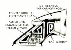
FIG. 3-PHANTOM VIEW of the Alpha-3 active AM/FM automobile receiving antenna.
