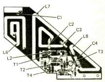
FIG. 5—PC BOARD showing location of all parts for the Alpha-3 auto radio antenna.
