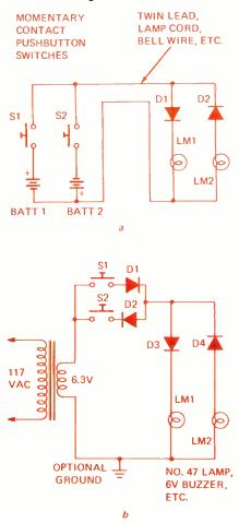
FIG. 3-PUSHBUTTON SWITCHES control the battery-operated (a) and line-powered (b) selective signalling systems.
