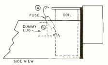
Whenever you service an early-run model 19P86 receiver, this modification should be added to the remote receiver. Fix-kit No. 966529, consisting of the fuse, a 1-point dummy lug, nut and screw, is available from the factory.
