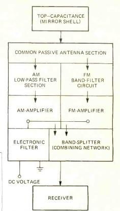
FIG. 4—BLOCK DIAGRAM of the Alpha-3. AM and FM signals are separated, amplified and recombined before going to the receiver.
