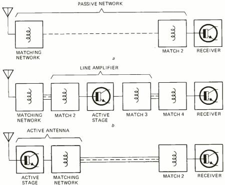
FIG. 1-THREE BASIC ANTENNAS. The simplest (a) is not amplified. Often a line amplifier (b) is between the antenna and the set. Active antenna (c) has a built-in integrated amplifier.
