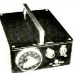
Transistorized Test Unit substitutes the tuner in defective TV Receiver to prove whether original tuner is good or bad.
