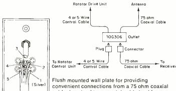
convenient connections from a 75 ohm coax cable downlead to a coaxial cable lead for a TV FM set, also from a rotator cable to a rotator control unit. Rotator outlet plug and co-ax connectors included.
