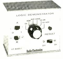
when the input is 1 and a 0 out when the input is 0; or it could *complement* the input, and put a 1 out when the input is 0and a 0 out when the input is a 1.
