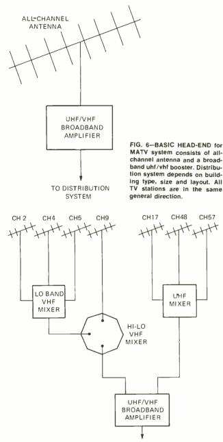
FIG. 7-SINGLE-CHANNEL ANTENNAS are needed when TV transmitting antennas are all in different directions from receiving site.
