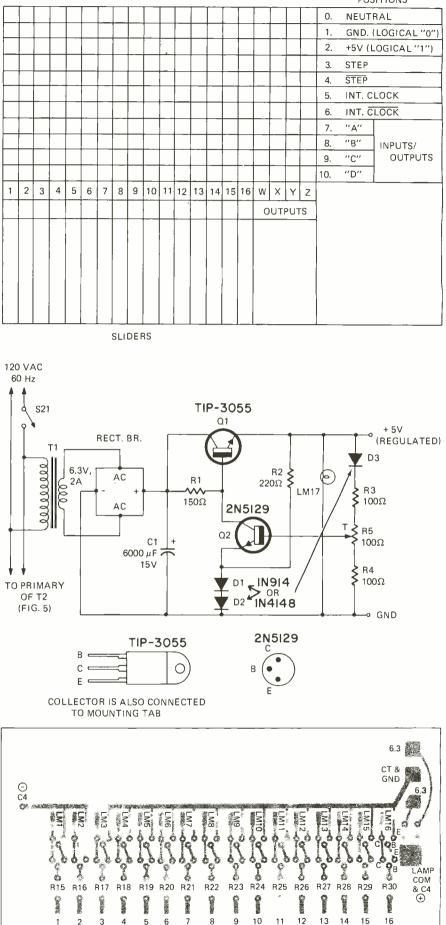
THESE DRIVER INPUTS ARE CONNECTED TO THE CORRESPONDING NUMBERED SLIDERS ON THE MATRIX SWITCH.
