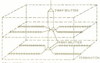
FIG. 3—TYPICAL LAYOUT OF MATV CABLE and tap-offs in long, low rambling buildings such as schools and motels.
