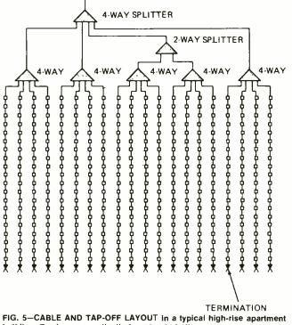
FIG. 5—CABLE AND TAP-OFF LAYOUI in a typical high-rise apartment building. Feeders run vertically from top to bottom.
