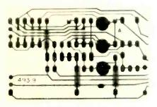
About fifteen of the small boards can be lined up on a single  $14 \times 17$  inch sheet of X-ray film. One X-ray picture shows both sides of the board. The large negative can be cut apart so shots of the individual boards can be enlarged and printed. The wiring and components become clear as shown.—Arthur B. Cecil, Jr.
