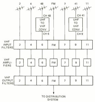
FIG. 9-FOR BEST UHF RECEPTION use a single down-converter with output on unused vhf channel for each desired uhf station. tennas are mixed and fed into a broadband amplifier. Broadband amplifiers have their limitations, however. Fig. 8 shows the type of head end that would be used for a large system where many channels were available.
