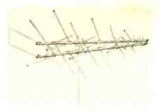
6- to 8-dB gain on most commonly used uhf channels. FM gain is 5 dB. The *J*-283X
