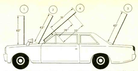
FIG. 6—WHIP ANTENNAS for automobile radios are usually mounted in one of four possible positions. The antenna on windshield post (4) is seldom fully extended to 39 inches and is usually pulled out to between 26 and 33 inches. (continued on page 88)
