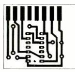
FIG. 2-FULL-SIZE FOIL PATTERN above is the circuit board you need for your own logic demonstrator. Use this pattern as is.
