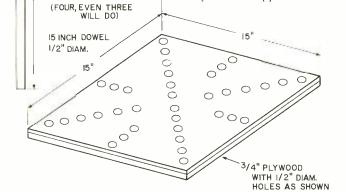
expensive and take up a lot of space. The drawing shows a simple support that I have developed for servicing round magnifying (shaving) mirror provides a view of the underside.-Charles R-E W. Nelson
