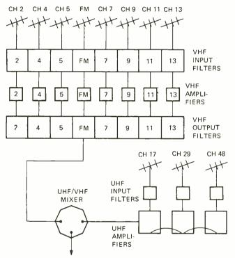
FIG. 8—HEAD-END ARRANGEMENT for uhf/vhf and FM reception. Uhf and vhf channels are received and amplified separately and then comblned in a mixer that feeds the distribution system.
