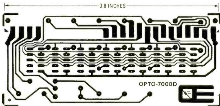
FIG. 7—DISPLAY BOARD foil pattern. You may want to make several and adapt them for use in other digital instruments using the FND357 or similar 7-segment LED displays.
