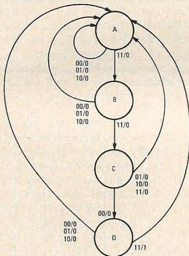
FIG. 25—STATE DIAGRAM of circuit with multiple inputs.
