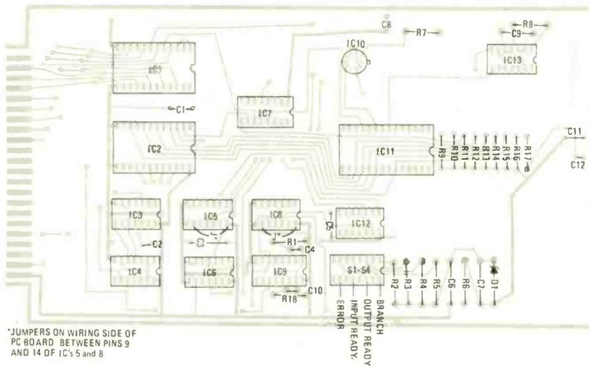
FIG. 10—COMPONENT PLACEMENT DIAGRAM shows where the parts go on the circuit board.
