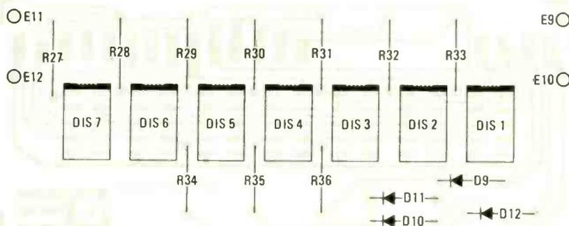
FIG. 8—COMPONENT SIDE of the display board. Leads through pads E9—E10 and E11—E12 form right-angle bracing when display board and main board are mated.
