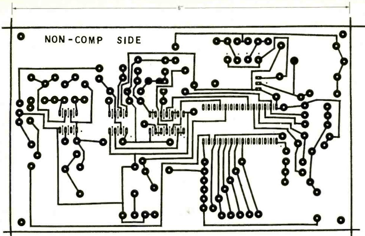
FIG. 3—FOIL PATTERN for the single-sided printed-circuit board.
