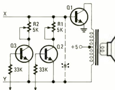
FIG. 3—TUNE MAKER CIRCUIT showing transistor on-off switches.
