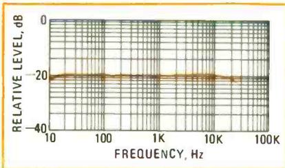
For the slower 3 3/4 ips speed, the maximum recording-output level obtainable at 10 kHz was approximately 14.0 dB below the mid-frequency maximum output level. These values are considerably better than those usually obtained when this tape is used on other decks, and underline the advantages of Tandberg's new recording electronics.
