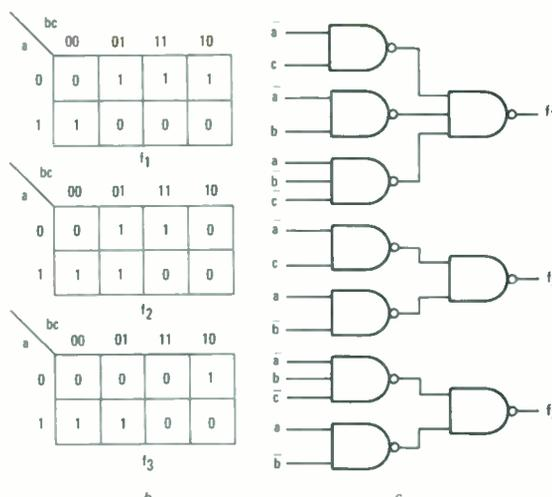
FIG. 17—MULTIPLE INPUTS AND OUTPUTS can also be handled. Truth table with three inputs and three outputs is shown in a. Resulting Karnaugh maps are shown in b; logic circuit is shown in c.
