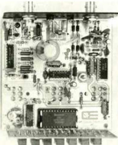
**INTERIOR VIEW** shows the component side of the frequency counter's main PC board.
