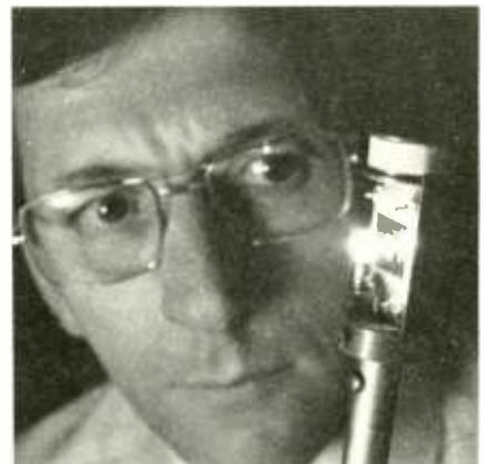
BELL LABS SCIENTIST prepares to test experimental two-layer gallium arsenide/aluminum gallium arsenide semiconductor crystal (shown to the right of the light). New crystal technique increases the speed at which electrons move through the crystal. Such a breakthrough in solid-state technology could lead to faster, more efficient semiconductor devices.
