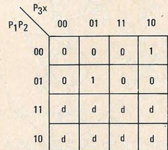
FIG. 34—KARNAUGH MAP for J-input of flip-flop FF1.
