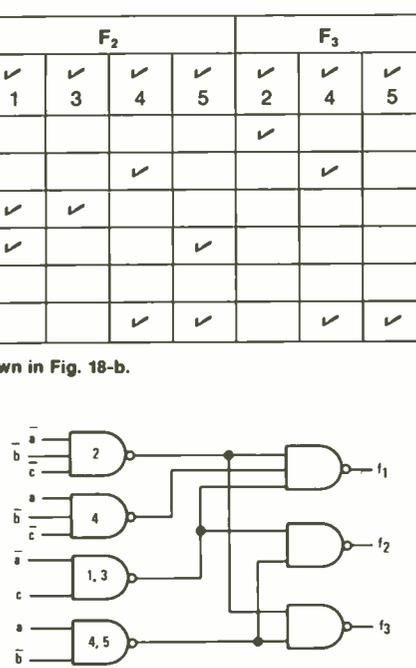
FIG. 21—SIMPLIFIED LOGIC CIRCUIT for three inputs and three outputs requires less gates than circuit shown in Fig. 17-c.
