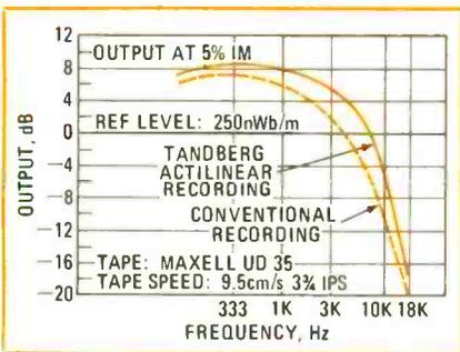
ing benefits provided by Tandberg's actilinear recording system, and also indicates the added dynamic range available at the slow 3 3/4-ips speed at all frequencies from 333 Hz up. In Fig. 4, the 0-dB reference level is taken as 250 nanowbers per millimaxwell, or approximately 2.6 dB above the standard NAB reference record level. Results of our lab measurements are shown in Table 1.
