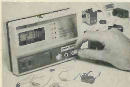
DETERMINING VALUES of ordinary capacitors is only one of the many uses of these versatile meters, such as the model 830 shown above from B&K—Precision, Dynascan Corp.
