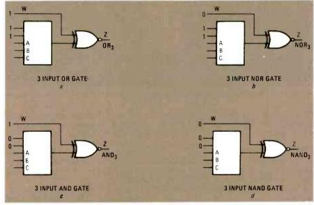
FIG. 5-VARIOUS 3-INPUT logic gates can be formed from a 5-input majority-logic gate.
