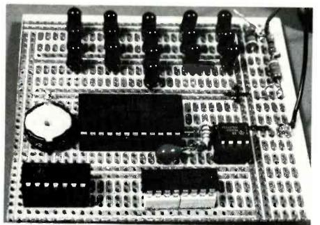
FIG. 47—TRIMMER PCTENTIOMETER at left of 74154 IC varies rate at which LED's flash. Mount board so LED's are visible through opening(s) in skin of robot.
