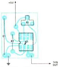
FIG. 52—INTEGRATED CIRCUIT, IC1, is a 555 timer (shown at lower-left in Fig. 50). One-kHz clock signal is fed to second PC board.
