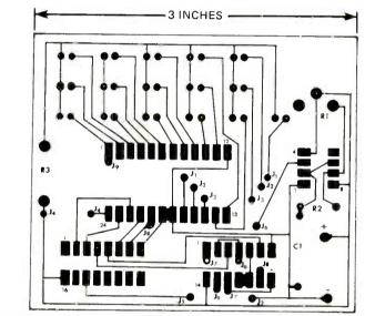
FIG. 48-PC BOARD for sequential-flasher circuit shown in prototype-version above.
