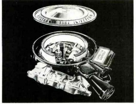
FIG. 3—CHRYSLER'S ELECTRONIC FWEL-INJECTION system rep.aces the carburetor with a complex pod of electronics, sensors and electromechanical devices.
