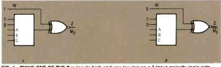
FIG. 4-TYING ONE OF THE five inputs high and one low leaves a 3-Input majority-logic gate.
