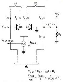
FIG. 7---CURRENT MIRROR PRINCIPLE is illustrated in CA3080 transconductance amplifier.
