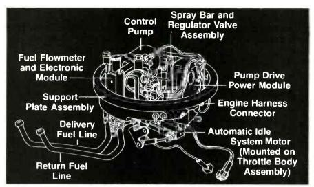
FIG. 4—THE AIR-CLEANER AND THROTTLE-BODY assembly in Chrysler's Electronic Fuel-Injection system contains the fuel-control pump and power electronics, fuel-flow sensing, pressure-regulating valves, spray bars, and automatic idle speed motor.
