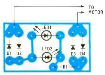
FIG. 44—PC BOARD for motor-direction indicator was designed for rectangular LED's. Circular ones will need their leads bent a bit.
