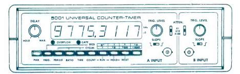
FIG. 2-TYPICAL UCT FEATURES are exemplified by front panel of Global Specialties' model 5001.
