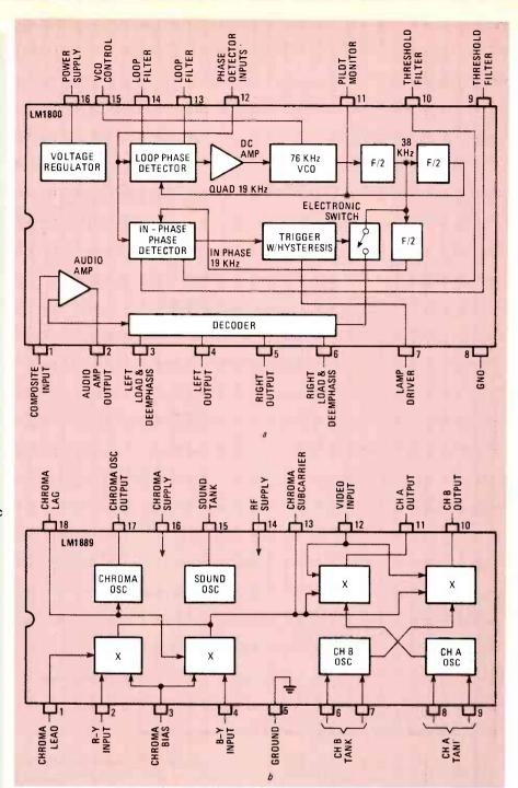
FIG. 2—ALTHOUGH DESIGNED for other purposes, the LM1800 and LM1889 can be used in decoding applications.
