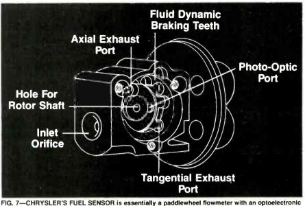
FIG. 7—CHRYSLER'S FUEL SENSOR is essentially a paddlewneel nowmeter with an optoelectronic interrupter providing a pulse rate proportional to fuel-flow rate.
