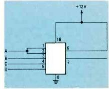
FIG. 9—MAKING TWO INPUTS into one gives that input twice the importance of the others.
