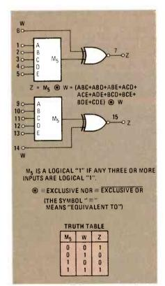
FIG. 2—THE MC14530 consists of two 5-input majority-logic gates, each followed by a NOR gate.
