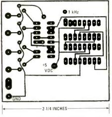
FIG. 53—DIVIDER CHAIN AND LATCHES are located on separate PC board.
