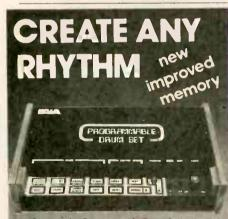
Our popular Programmable Drum Set's simple programming system allows even first time users to structure bass, tom, snare, wood-block and clave sounds into any rhythm in any time signature. Versatile memory organization provides simultaneous storage of two separate rhythm patterns each with its own bridge rhythm. Bridges are activated from either the control panel touch plate or optional foot switch and are automatically synchronized to the main rhythm.
