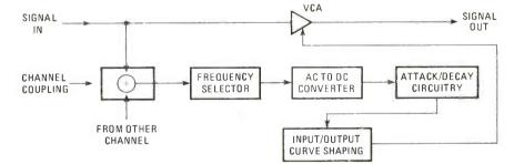
FIG. 1-DYNAMIC RANGE EXPANDERS use a VCA to "ride gain" on the incoming signal.
