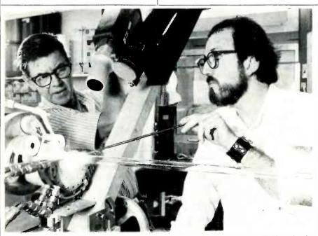
THE ULTRATRANSPARENT GLASS FIBERS that will carry light signals to and from the three Southern Bell switching offices in Atlanta are fabricated by a process that begins with a silica tube being heated on a glass lathe.
