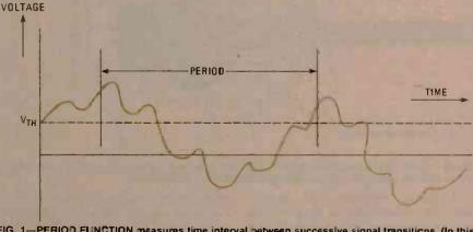
FIG. 1—PERIOD FUNCTION measures time interval between successive signal transitions. (In this example, threshold voltage  $V_{TH}$  defines the transition-point.)
