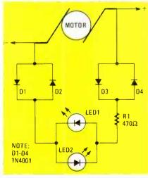
FIG. 42—MOTOR-DIRECTION INDICATOR uses twelve volts. Diodes and resistor reduce voltage and current to safe levels for LED's.
