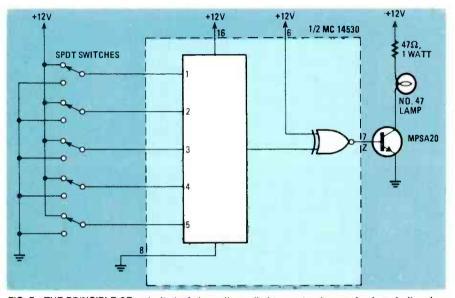
FIG. 7-THE PRINCIPLE OF majority logic is easily applied to a vote where a simple majority rules.
