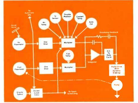
FIG. 8—SIGNAL PROCESSING in Chrysler's EFI system. Block diagram gives you some idea of the complexity of the system. The air and fuel one-shots are of opposite polarity, resulting in a continuously variable net charge on the integrator and extremely fine control of the duty cycle of the drive pulse to the pump-control transistors.
