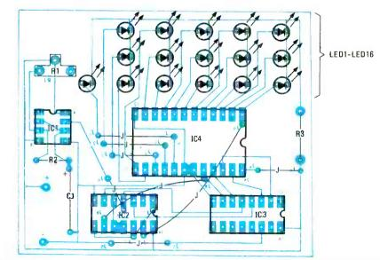
FIG. 49—NINE JUMPER WIRES are required on sequential-flasher board. "Odd" LED at left can be ommitted without upsetting anything if symmetrical layout is desired.
