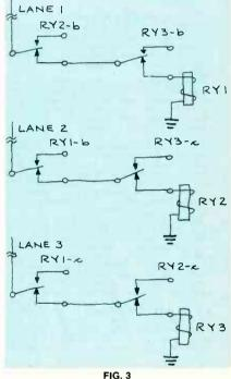
of relay RY2 is not completed because the RY1-a contacts are now open. Thus, relay RY2 does not energize and contacts RY2-a stay open. Since contacts RY2-a are open, lamp L2 does not stay on-it only flashes briefly when the Lane-2 switch is hit.
