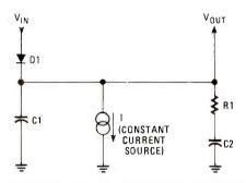
FIG. 5—TWO-STAGE attack/delay circuit is used by dbx for greater flexibility.
