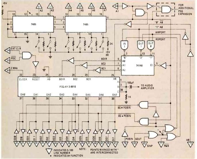
FIG. 9—TYPICAL INTERFACE for the S-100 bus. This design requires only an 8080 IN OF OUT instruction to read-from or write-to the PSG.
