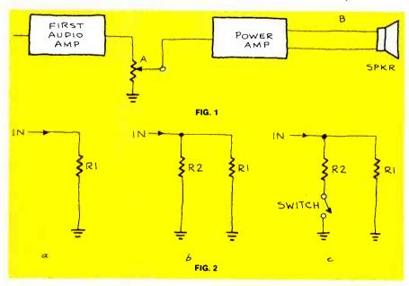
The block diagram in Fig. 1 shows two points in any amplifier where the audio signal is readily accessible. One is the volume control (A) and the other is the output to the speaker (B). For our purposes, we'll consider points A and B to be the same.
