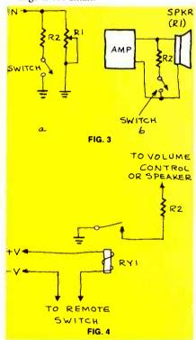
So far so good—we have changed the volume. However a switch on the amplifer doesn't solve the original problem and it is often unsatisfactory to run long audio lines around a room. That means that we must find some way to operate the switch by remote control.
