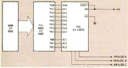
be tied directly to the microprocessor's data lines if decoding is provided to place the PSG in its "inactive" mode (see Table 1) when the PSG is not being accessed.
