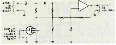
FIG. 5-COMBINED LOW-FREQUENCY EQUALIZATION and cone-displacement signal-modifier circuits.
