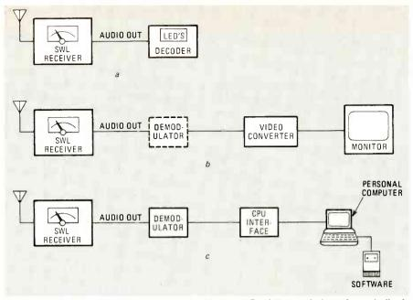
FIG. 2—THREE common systems for decoding Morse and Baudot transmissions electronically. A demodulator or terminal unit is often required in system b.
