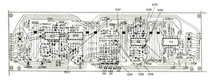
FIG. 16—PARTS PLACEMENT guide for the front PC board. The use of IC sockets is recommended.
