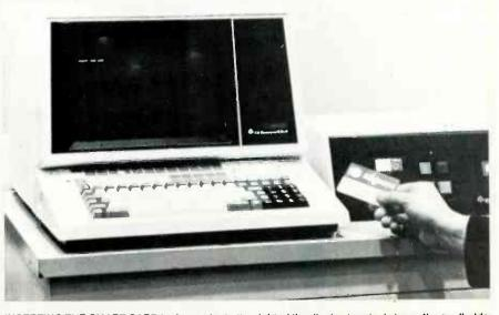
INSERTING THE SMART CARD in the reader to the right of the display terminal shows the cardholder his bank balance. It also supplies any other information for which the system may be programmed, or may transfer funds according to his instructions.
