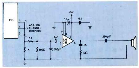
FIG. 7-THIS circit sums the PSG's three analog channels, amplifies them, and drives a speaker.
