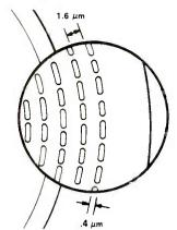
MICRO PITS IN THE SURFACE of the videodisc carry the encoded video and audio information.
