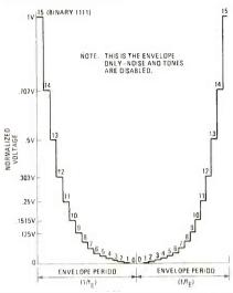
FIG. 4—OUTPUT LEVELS for all possible combinations of bits B0-B3. Writing 0000 on bits B0-B3 turns a channel off.
