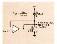
FIG. 12—GATE-VOLTAGE DERIVER, IC7-d, is used to control gain of op-amps IC4 and IC5.
