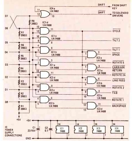
FIG. 3—FUNCTIONS PERFORMED by each IC section are clearly indicated. Bar over function description represents a logic-"low" output.
