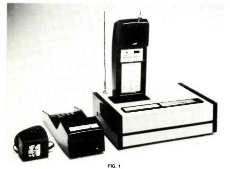
The handset contains a 1.7-MHz receiver with an internal rod antenna, a 49-MHz transmitter with a small telescopic (or optional "rubber ducky") antenna, a continuous 5.3-kHz pilottone oscillator, a function switch, and a Touch-Tone pad if the handset permits dialing out.
