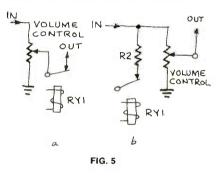
Increasing the volume only takes some minor changes in the circuit of Fig. 4. The relay connection is shown in Fig. 5-b. In this case, the volume is set at normal with R2 in the circuit. Energizing the relay removes R2 from the circuit and the full signal goes to the volume control and out.
