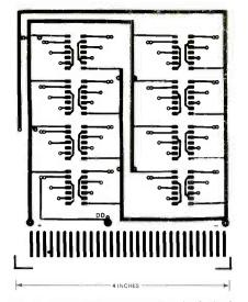
FIG, 81—IF "DROP-DEAD" feature is desired, "double-donut" pads must be jumpered together.
