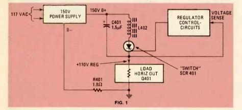
ply is held constant at all times, all of the outputs (high voltage, sweep, boost, and the flyback-derived low-voltage DC supplies for the rest of the set) are held at the correct level.
