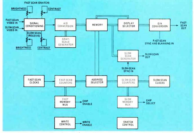
FIG. 1—LOGIC AND TIMING portions of Picture Phone circuit are shown at bottom of block diagram; video-processing blocks are at top.
