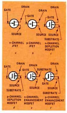
FIG. 5—THE DIFFERENT KINDS of FET's are identified in schematic diagrams by these standard symbols. Note that the depletion devices shown in *c* and *d* are also known as enhancement/depletion MOSFET's (see text).
