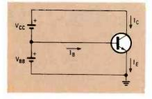
FIG. 2—THE VOLTAGE POLARITIES required to turn a bipolar NPN transistor on, as well as the currents that are produced. This circuit is used as an illustration only; do not attempt to build it, as it would most likely destroy the transistor.
