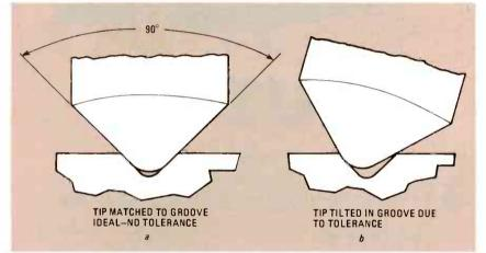
FIG. 2—THE STYLUS TIP must not be tilted left or right with respect to the record groove as shown in *a*. When stylus tip is tilted, proper contact with the record groove does not occur, as shown in *b*. This tilt angle is sometimes referred to as angular tolerance.
