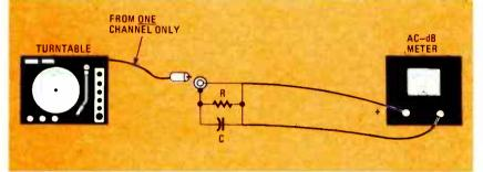
FIG. 10—TEST SETUP for measuring the frequency response of a phono cartridge at the output of the cartridge. The R-C load impedance network is connected across the output terminals of the cartridge.
