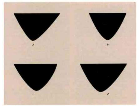
FIG. 4—BIRADIAL TIPS include several different shapes. The Shibata tip is shown in *a*, the Pramanik is shown in *b*, the quandrahedral is shown in *c*, and the hyperbolic is shown in *d*.
