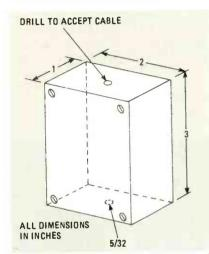
FIG. 4-THE AIR TEMPERATURE sensor is mounted in a box with these dimensions and mounted outdoors.
