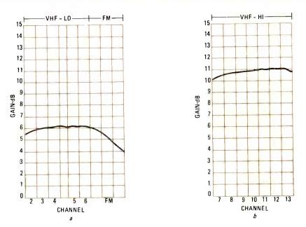
FIG. 12—THE GAIN OF THE ANTENNA SHOWN IN FIG. 5. The gain for the low band (channels 2-6) is shown in *a*; the gain for the high band (channels 7-13) is shown in *b*.
