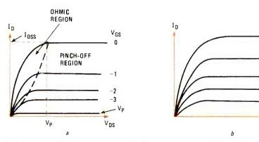
FIG. 6—DRAIN CHARACTERISTIC CURVES for the various types of FET's are shown here. The curves for a JFET are shown in *a*; the curves for enhancement and enhancement/depletion MOSFET's are shown in *b*.
