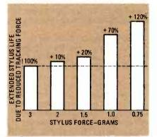
FIG. 6—AVERAGE TIP LIFE increases dramatically as the tracking force is reduced.
