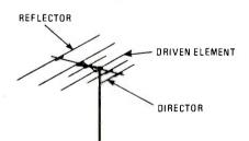
FIG. 4—A SIX-ELEMENT VHF antenna such as this is good for local TV reception.
