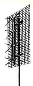
FIG. 7—HIGH GAIN AND LOW COST are among the reasons for this UHF antenna's popularity.
