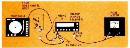
FIG. 11—TEST SETUP for measuring the frequency response of a cartridge with the cartridge connected to a preamplifier. In this case, the load impedance is the impedance of the phono input of the preamplifier. A "Y" connector is used to connect an R-C circuit across the output terminals of the cartridge if the load impedance needs to be altered.
