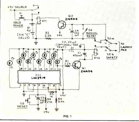
ing. Assembly is very easy (incidently, I'm only 13 and had very little trouble with it). As I said, with the values shown, the timing period is about 10 seconds; however, nothing in the circuit is very critical. Lead lengths should be kept as short as possible, however; if they get too long, oscillation may occur. To prevent that, C2 can be installed in the circuit as shown.
