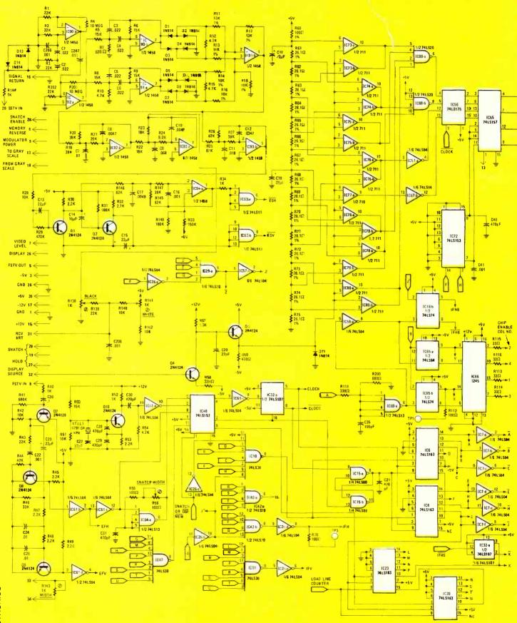
FIG. 2—HEART OF THE PICTUREPHONE is its memory, sixteen 4K-bit IC's that store video information prior to scan conversion.
