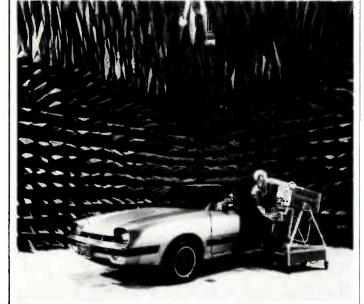
THE ABSORBING WEDGES, CONES, OR PYRAMIDS in this room make it look exactly like an acoustic anechoic chamber. Actually the cones are made of material designed to be especially absorptive to radio waves in the range of 14 kHz to 1 GHz. The chamber was installed by the Ray-Proof Division of Keene Corp. of Norwalk, CT.
