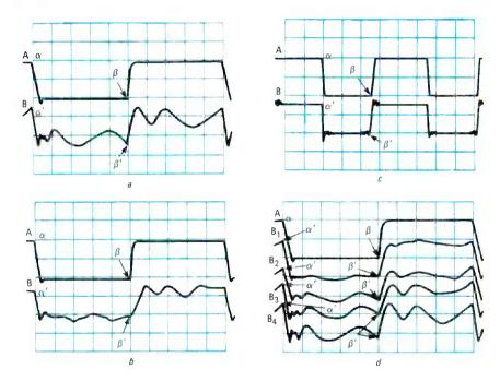
FIG. 4—ORIGINAL AND IMAGED signals for three different frequencies: 1 MHz (*a*), 0.8340 MHz (*b*), and 0.3579545 MHz (*c*). Fig. 4-*c* shows images probed at 100, 200, 300, and 400-meter points.
