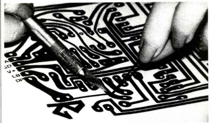
**Part 2** LAST TIME, WE SHOWED you a step-by-step method for developing a PC-board layout from your working prototype circuit. The first thing we'll do this month is finish that layout.
