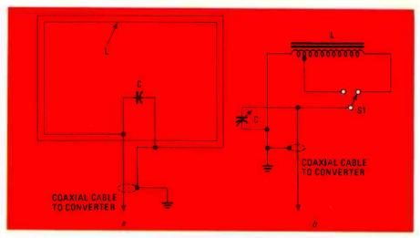
FIG. 4-OPEN-LOOP ANTENNA is shown in a; ferrite loop at b.
