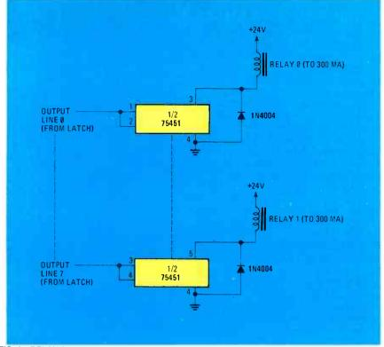
FIG. 8-RELAY DRIVER example.
