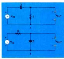
FIG. 7—A PASSIVE HIGH-PASS FILTER is shown in a, a low-pass filter in b.
