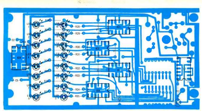
FIG, 5—PARTS PLACEMENT on "component-side" of display board. Note that foil pattern shown is on side of board *opposite* the one on which components are mounted.
