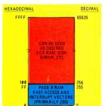
FIG. 3—MEMORY ARCHITECTURE of 8080 and Z80 microprocessors.
