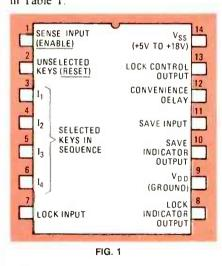
Figure 1 shows the pinout of the LS7220, and Fig. 2 shows a block diagram of the IC.
