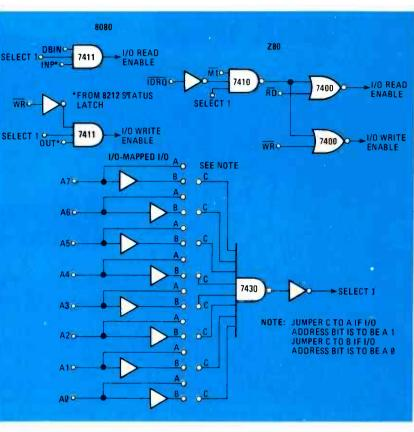
FIG. 4-1/O DECODE for the 8080 and microprocessors.
