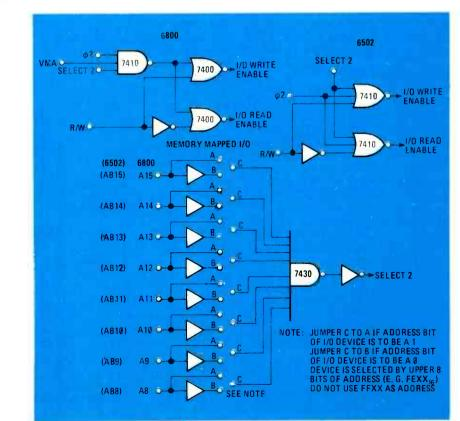
FIG. 5-I/O DECODE for the 6800 and 6502 microprocessors.
