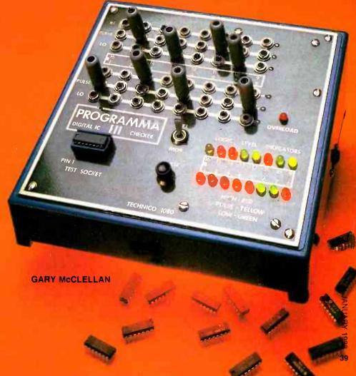
cover that there are only seven IC's in the whole unit! They are all standard, lowcost parts, which makes them easy to find. In addition, this is probably one of the first projects you've seen that uses a VMOS power FET. It does a superior job in the pulse-generator section, and allows pulses to swing the full five-volt range. The display electronics mount on a separate PC board, and simply plug into the panel-board, further simplifying construction.
