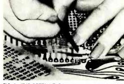
FIG. 6—IT IS OFTEN HELPFUL if you identify IC pin numbers, edge connectors, and the like for later reference. Using transfer type for that, as shown, can give your project a professional appearance.
