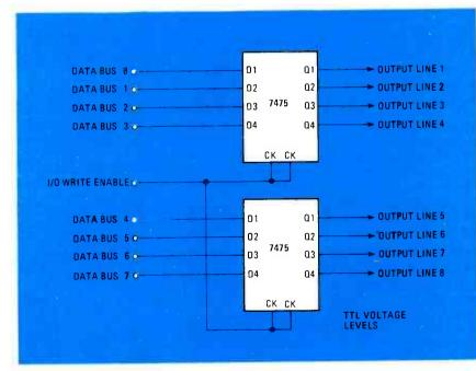
FIG. 7.-DISCRETE I/O write logic.
