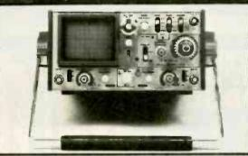
V-509 Delayed Sweep DC-50 VHz **Mini-Portable Dual Trace**
