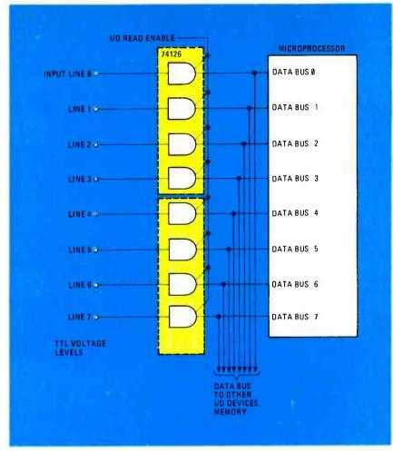
FIG. 6-DISCRETE I/O read logic.
