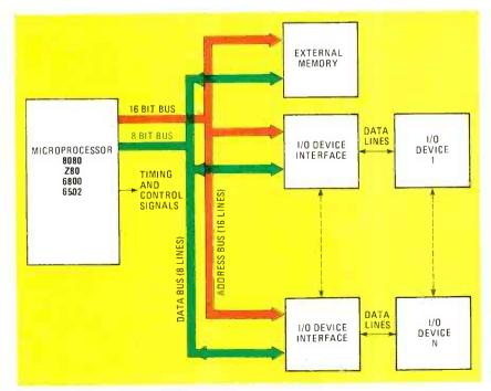
FIG. 1-MICROPROCESSOR system structure.
