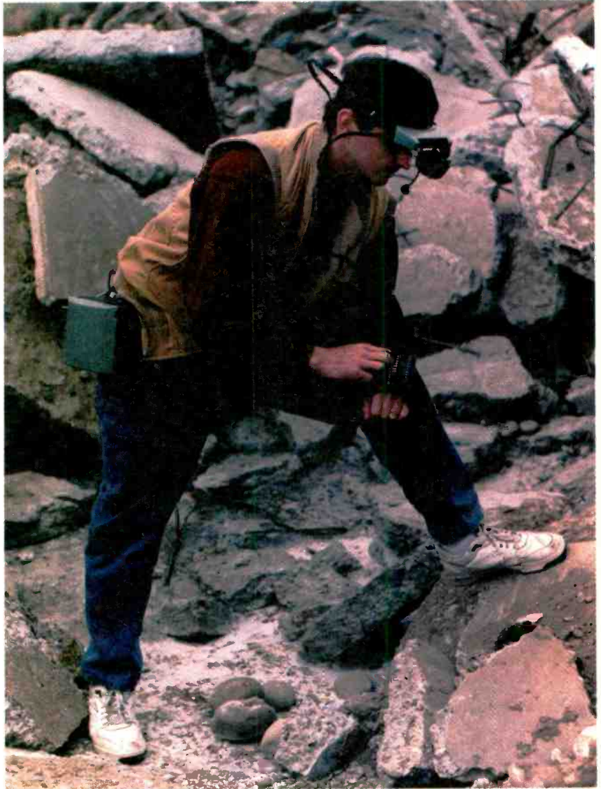
HERE AN INVESTIGATOR WEARING THE TEAM LEADER computer on a waistband enters information on a wrist-worn keyboard. A small display screen and microphone is worn on the headband.
