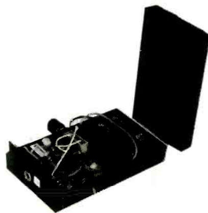
The small size of the Airport Buddy's PC board lets the entire unit fit into a small case that can be easily carried in a shirt pocket. Here is the author's prototype. Note that ANT1 is simply a length of insulated wire.
