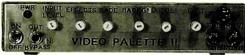
Fig. 4. Because the Video Palette II uses simple control signals, no high-frequency signals need to leave the PC board. That feature lets you design the front panel to your own requirements. Here's the front-panel design that the authors used on the prototype.
