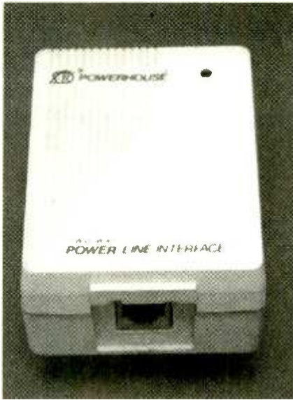
Fig. 4. Command interfaces for the X-10 protocol are small, inexpensive, and reliable. This particular unit has the ability to receive feedback from the other modules and send it back to the main controller.
