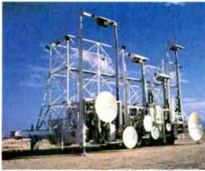
BICOMS, THE MOBILE RADAR UNIT—40 feet tall, 66 feet long, 37 feet wide, and weighing 90 tons—is shown here at Holloman Air Force Base, New Mexico.
