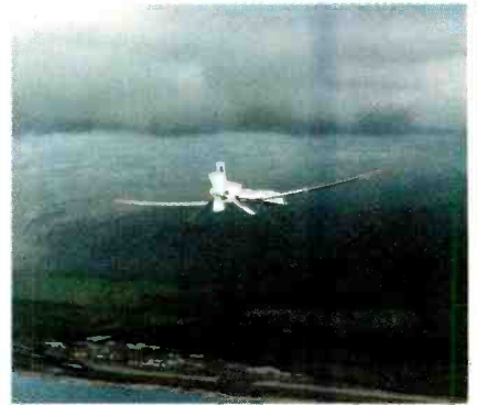
THE ALTUS ROBOTIC AIRCRAFT measures solar energy that is transmitted and reflected by cirrus clouds in the Hawaiian islands.
