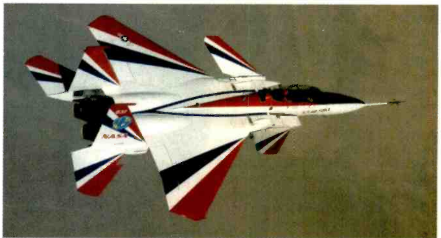
A HIGHLY-MODIFIED F-15 AIRCRAFT UNDERGOING TESTS at NASA's Dryden Flight Research Center, Edwards, CA, to evaluate how the neural network software will enable aviators to control and safely land disabled airplanes.
