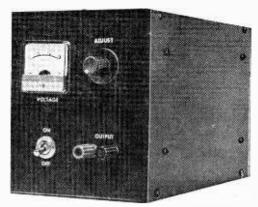
Output and control panel of this compact, utilitarian, low-voltage, regulated power supply usable either in experiments or as primary supply for operating equipment.
