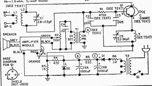
L3 is then self-supporting when mounted directly to C5. Use a rubber grommet to protect the leads from L3-C5 as they pass through the chassis from bottom to top.
