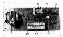
All circuitry, including AC power supply, is assembled on printed circuit board. Photo shows location of most major components.
