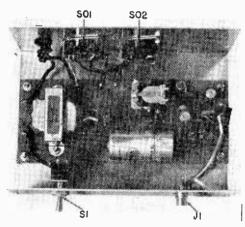
Completed PC assembly fits easily in base of  $3 \times 5 \times 7$ -in. aluminum cabinet. Use at least #18 wire to connect up SO1 and SO2.
