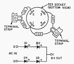
Fig. 1. Above and right, two ways to use silicon diodes to replace obsolete 5Z3 rectifier. All diodes are 800 PIV, 1 A types; resistors R1, R2, R3, and R4 at right are 470k, ½-watt units; resistors R5 and R6 are 1-ohm, 2-watt units; capacitors C1, C2, C3, C4 are standard .001-uF, 1000-V ceramics.
