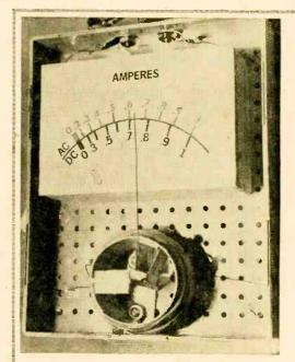
Basic structure of moving-vane ammeter is shown in photo above and in detail drawing at right. Text describes how unit is calibrated for both AC and DC readings.
