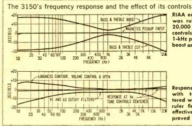
RIAA equalization on 3150 was ruler flat from 20 to 20,000 Hz. Bass and treble controls had fulcrum around 1-kHz point, with maximum boost and cut of some 20 dB.
