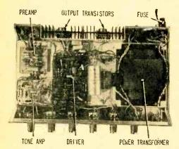
Each side of chassis contains printed circuit modules for single amplifier channel (this is upper side of completed amplifier). Topside also contains power-supply filter, shown to left of husky power transformer. Even chassis is assembled in modular form: front (with controls), back, and amplifier base.
