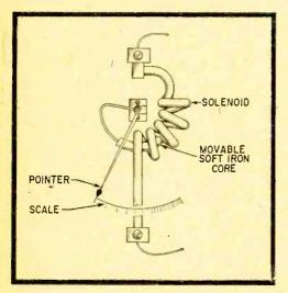
Commercial moving-vane ammeters of yester-year were much like water meters. Note that device was accurate only if vertical.
