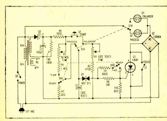
on (and the bridge conducts) whenever a current of more than 200 microamps (1/5 of a milliamp) is fed into the gate terminal.
