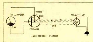
Liquid photocell produces output of several milliamperes proportional to intensity of light shining on it (the more light, the more current). Cell can be rejuvenated by renewing cuprous oxide on the copper surface.
