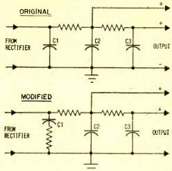
Try a resistor in series with input capacitor C1. Try various values until the output voltage is correct. The resistor will probably have to be a wire wound type rated at 10 watts or more.
