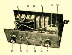
View shows front panel and interior layout of timer assembly. Notice how C1 and C2 are taped together and comented in position on rear panel. With exception of variable resistors, all semiconductors and resistors are placed on an insulated tie strip, to which tie strip terminals have been staked. Strip is mounted adjacent to power transformer on bottom of cabinet and raised by spacers to prevent shorting out circuitry.
