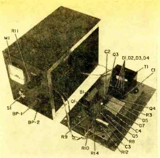
Here's what's inside our regulated supply. Note accessibility of components on circuit board. Because power transformer is relatively heavy, it needs extra support to prevent board from cracking.
