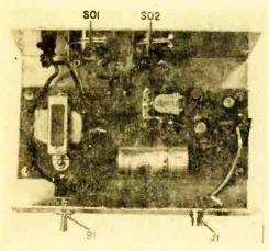
Completed PC assembly fits easily in base of  $3 \times 5 \times 7$ -in. aluminum cabinet. Use at least #18 wire to connect up SO1 and SO2.
