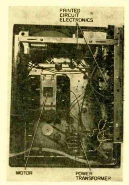
Thanks to use of printed circuits, underside of Tandberg is clean and uncluttered.
