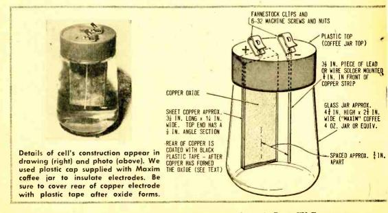
is not critical, but the jar must be made of clear glass and should have a plastic lid, or you will have to make a wooden or plastic lid to fit. The copper sheet may be difficult to obtain. We cut and flattened a length of ½-in, copper tubing for our model.
