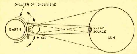
During an eclipse, solar X-rays that reach the earth's ionospheric D-layer are modulated by the moon. X-ray intensity decreases at A, minimum at C, and increases at B.
