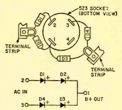
Fig. 1. Above and right, two ways to use silicon diodes to replace obsolete 5Z3 rectifier. All diodes are 800 PIV, 1 A types; resistors R1, R2, R3, and R4 at right are 470k,  $\frac{1}{2}$ -watt units; resistors R5 and R6 are 1-ohm, 2-watt units; capacitors C1, C2, C3, C4 are standard .001-uF, 1000-V ceramics.
