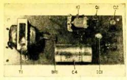
All circuitry, including AC power supply, is assembled on printed circuit board. Photo shows location of most major components.
