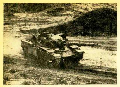
Fitted with laser simulator on top of gun barrel, British-made Chieftain tank rumbles into battle on training exercise. Tank's engine, radio, and gun go dead when hit with electronic shells; smoke automatically pours from tank when hit would have left it totally disabled.
