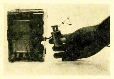
Though no instructions are furnished, relay within ColorVolt can be removed if unit is to be operated with loads under approximately 150 W. Effect is to cause regulator to operate on continuous-duty cycle. Alternatively, simple spst switch can be installed.
