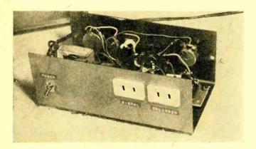
Rear view of timer assembly showing locations of two outlets where power cords for audible indicator for both process timer and enlarger are plugged in. Right-hand outlet is connected to short duration timing circuit for enlarging; left-hand outlet is connected to long duration timing circuit for processing. Bell or buzzer is powered through latter outlet.
