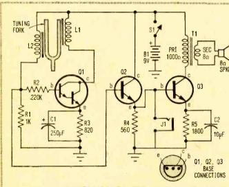
Schematic reveals Freq Standard's simple but highly accurate circuit. Mechanical tuning fork controls Q1's frequency of oscillation; audio tone appearing at Q1's base is then amplified and fed to either J1 (for further amplification) or direct to Freq Standard's speaker.
