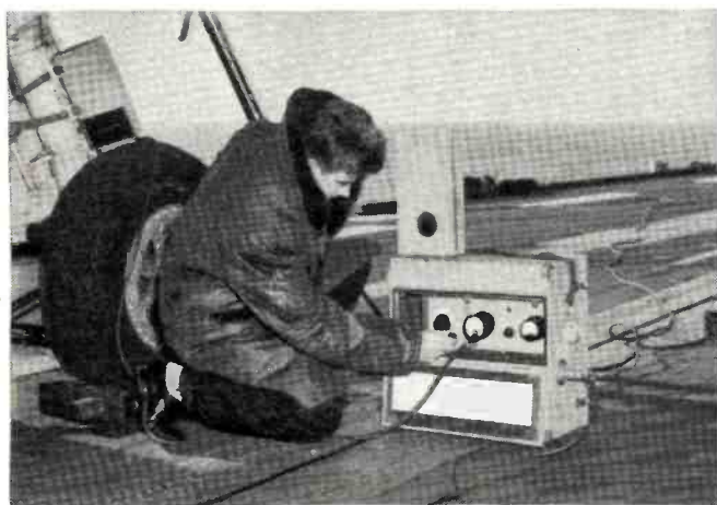
Fig. 8. A v.h.f. direction finder on an aircraft carrier deck.
