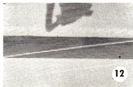
Fig. 12. In this case, sync signals are only slightly darker or stronger than blanking and dark-picture signals. This trouble is caused by excessive signal input and consequent limiting action in the video amplifier due to incorrect setting of a.g.c. threshold adjustment. Fig. 8 (Part 1) shows the result of same condition on test pattern. Dark objects at top of this picture are legs and shadow of home-plate umpire.
