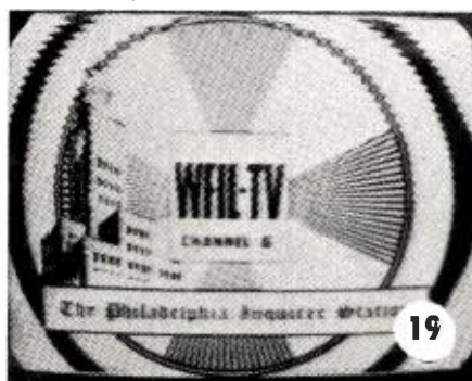
Fig. 21. Horizontal pulling and unstable horizontal sync may result from certain conditions of reflections or ghosts. Ghost signal in this example is almost merged with direct signal, resulting in poor picture quality and horizontal pulling. Occasionally, when intensity of a close-in ghost is approximately the same as direct signal, the two may alternate in taking control of horizontal oscillator. In such cases, picture shifts erratically a distance equal to spacing between the ghost and direct signal.
