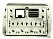
continuously variable a-f source, calibrated amplifier and channel analyzer, electronic circuit tester, and an impedance indicator. Net price \$345. Radio Corp. of America, RCA Victor Division, Camden, N. J.—RADIO & Television RETAILING
