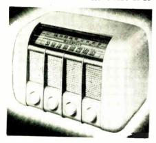
superheterodyne; two bands for shortwave and broadcast. Sensitive R.F. stage for distant reception. Built-in loop aerial, full range tone control; illuminated slide rule dial. Ivory-finished plastic cabinet. 6" oval permanentmagnet dynamic speaker. Size: 111/2" x 75/8" x 63/4"
