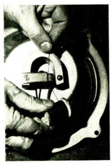
A When the armature of a magnetic speaker does not vibrate freely, this may be due to dust or rust between armature and pole pieces. A strong thread may be inserted as shown, and used to clean out the foreign matter.
