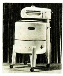
130, shown here, has a large, extra-capacity tub of triple-baked porcelain with splashproof rim; a chassis of monosteel construction with stamped steel base and legs welded into a single rigid unit; fully enclosed wringer column; controls located on the wringer head; and a standard-make, full ½ h.p., rubber-mounted motor which includes a rubber-jacketed cord. Blackstone Corp., Jamestown, N. Y.—RADIO & Television RETAILING
