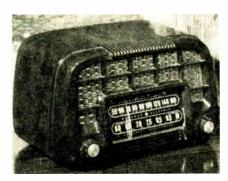
superheterodyne standard circuit: broadcast and short-wave bands. Tone control. One-piece molded plastic cabinet; deep recessed molding sets off well-lighted dial, with specially designed surface to give three dimensional look to numerals. Also available in ivory plastic (Model 219). Size: 131/4" wide, 8 1/16" high, 83/8" deep. Model 321, below, ac-dc 6 tube su-
