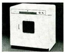
drying cycle; interior illumination, and ozone lamp. Average washer load of clothes will be damp-dried in approximately 20 minutes or less. Operates on 230 volts, 60 cycle, with current draw of 4600 watts. Dimensions: 36" high X 31" wide X 2634" deep (not including handle.)
