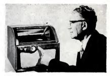
Edward Gray is shown starting his newlydeveloped Phono-Gard record player, which plays all 3 sizes of records without needle scratch. A transparent canopy isolates turntable and record, and the tone-arm moves from a locked and inaccessible position onto the record. No manual adjustment is necessary for record size. Player is excellent for demonstration playing and industrial programming.
