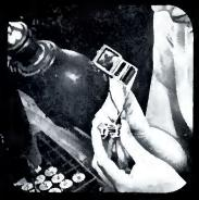
Completed mounts are inspected for visual defects.
