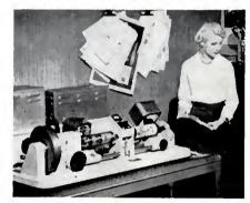
The Fairchild Scan-a-graver Cadet is a table-top machine which uses electronics, optics, and precision mechanics to make plastic half-tones automatically. Designed for the weekly newspaper and job shop, the Cadet makes a maximum eight inch by six inch 85-screen cut in 24 minutes.
