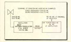
Fig. 1—Block diagram of a continuous type UHF tuner operating on channel 27 with a VHF tuner acting as first UHF i-f amplifier.
