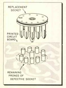
Fig. 1—Trimming the plastic around a broken printed circuit socket prepares it for easy replacement fitting. See text.
