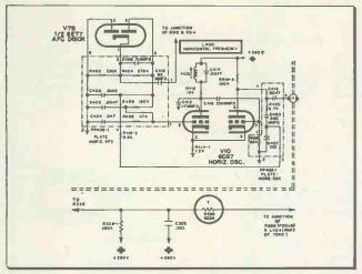
In Sylvania TV chassis 548-1, -2 code 04, the plate-horizontal afc and oscillator printed networks have been changed.
