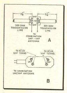
Fig. 2 (A)—Stub arrangement matches a single feedline UHF/VHF antenna combination to TV set and eliminates antenna switching. (B)—Commercially available cross-over net which is used for same purpose.
