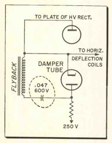
Fig. 4—A shorted .047  $\mu$ f capacitor was installed between plate and cathode of a damper tube, killing B + boost.
