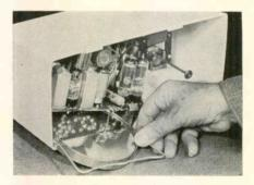
Fig. 2—A magnifying-type shaving mirror can be utilized in finding minute breaks in a printed circuit board.
