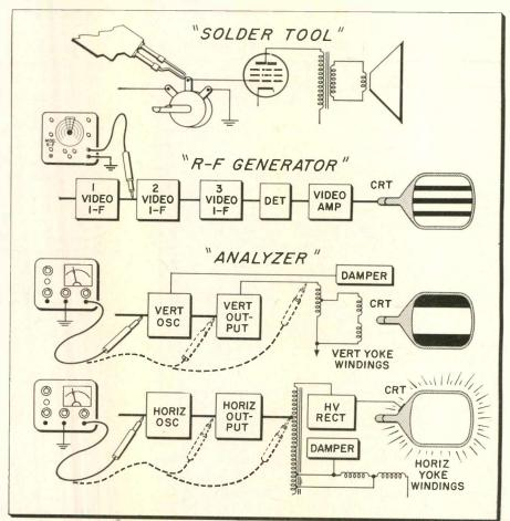
put tube's coupling capacitor was substituted with an open capacitor (the other Editors did not witness the "bugging"). Turning the set on, we naturally had no raster. Each instrument restored the raster when a horizontal signal was applied to the grid of the set's 6BG6 output tube.
