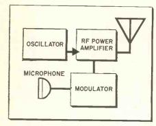
Fig. 1—Basic circuitry of typical marine type radio telephone transmitter.
