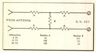
Installing a signal attenuator network in Fleetwood TV sets corrects an extreme overload condition.
