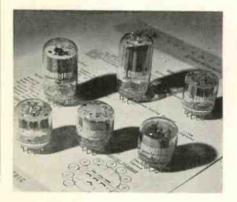
tional receiving tube plus two selenium diodes; 6K11 3-section triode, performs functions similar to those of the 12AU7 and 12AX7 conventional receiving tubes; and 6AX3 damper diode, operates similarly to the 6AX4GTB conventional receiving tube. General Electric Co., Receiving Tube Dept., Owensboro, Ky.
