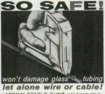
ARROW STAPLE GUNS can't damage wire or cable because driving blade automatically stops staple at right height! That's why Arrow Staple Guns are proved safer on jobs all over the country. And Arrow staples have tremendous holding power because they're rosin-coated, have diverging points that lock into wood.
