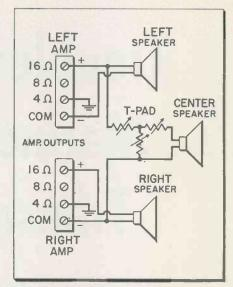
Fig. 4—Circuit for adding a third speaker operated from the sum of the two stereo signals. Action of each stereo amplifier is push-pull.
