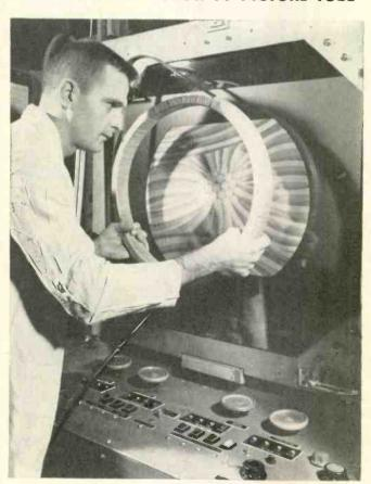
A rainbow of color is produced on RCA's new 21-inch color tube during one of many tests at the company's Lancaster, Pa. plant. Providing up to 50% brighter pictures with greater sharpness and contrast, the tube also enhances black and white images. Improved phosphors are largely responsible for advantages of the new tube.
