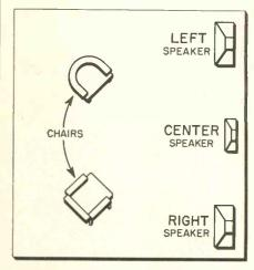
Fig. 5—Room lay-out using a third speaker from two stereo channels. Middle speaker can be relatively small but should respond well at mid and high frequencies.
