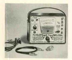
compact unit with a large 3" meter calibrated for direct reading of percentage of amplitude modulation on both positive and negative peaks. It has a direct reading scale for 0-5 watts r-f as well as a 0-400 ma r-f scale. Provides a high impedance input for use with Handy Talkies. A "T" pad attenuator is available as an accessory which adapts the model 510 for use with transmitters rated up to 50 watt input. Seco Electronics, Inc., 5015 Penn Ave. So., Minneapolis, Minn.
