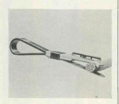
cally suited for the customary inside type ¾18", ¼", ¾8" or ½" cables, but will handle thin sheathed cable up to 1" diameter. Cuts are always ½2" deep. \$7.40. Also available, cable sheath slitter #N-62267 for slitting the cable lengthwise after circular cutting, \$4.20. P. K. Neuses, Inc., 511 N. Dwyer St., Arlington Heights, Ill. For more data, circle 5-73-3 on coupon, p.57
