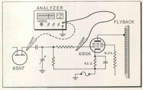
Fig. 2—Substituting an open coupling capacitor in the horizontal oscillator plate-to-output tube grid effected an open signal path, as shown. Using an analyzer instrument, a raster appeared when a pulse was applied at the 6BG6's grid, but didn't appear when applied at the 6SN7's plate. This isolated the defect between grid and plate.
