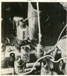
Fig. 3—Broken rear TV control shaft extensions can be repaired by using a heavy plastic knitting needle and wire.
