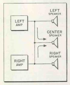
Fig. 2—Block diagram indicates a method of combining right and left channels at amplifier's output for center speaker operation. Center speaker can be either a sum or a difference signal.
