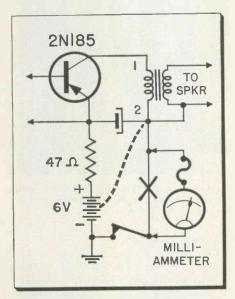
Fig. 1—In a Philco TR model T45-124, low battery life, weak volume and erratic operation were caused by the power supply "closing" at 3 volts instead of 6 volts.
