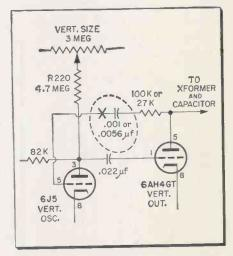
Fig. 2—A GE TV model 21C10's upper vertical compression was traced to a leaky plate-to-grid coupling capacitor.
