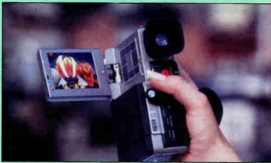
The Sony DCR-PC7 has a 2.5 inch LCD screen and color viewfinder that would allow a news reporter to shoot a stand-up solo.
