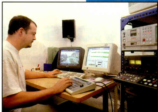
Mike Fraser Ltd uses the Studio Audio & Video Ltd SADiE hard disk system post sync in a sound suite without holding up the telecine.
