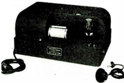
Test results are shown on drum in center
