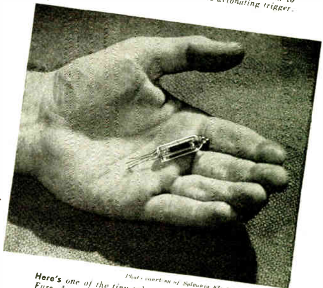
As target enters wave field, the waves are reflected back to the fuse where they release the electronic detonating trigger.
