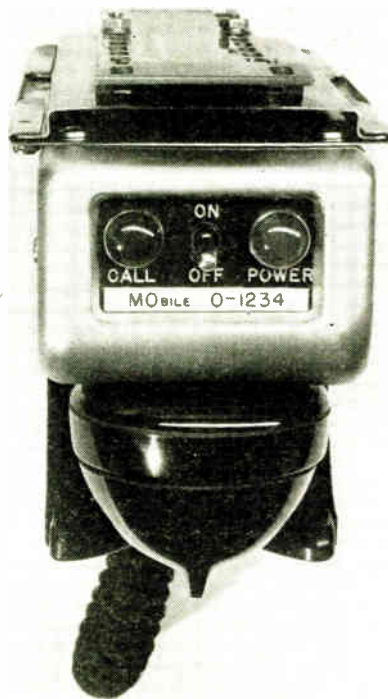
Control unit, mounted under dash and housing switches, indicator lamp and call bell
