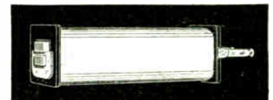
Coil core of a.c. relays is of thin laminations of silicon steel, riveted together. This reduces hysteresis and eddy current losses, gives large amount of power with small heat losses.
