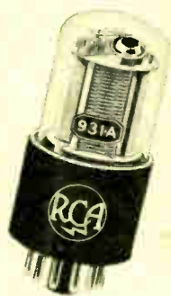
RCA-931-A. Current amplification is 1,000,000. Has S-4 spectral response. Maximum response at 4200 Angstroms. Range, approximately 3000 to 7000 Angstroms.
