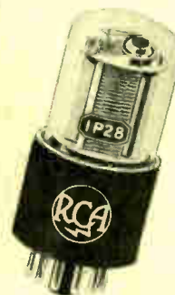
RCA-1P28. Current amplification is 200,000. Has S-5 spectral response. Maximum response at 2537 Angstroms. The tube has extremely low dark current.
