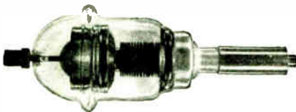
TYPE T—VACUUM VARIABLE CAPACITOR Peak Volts 10,000 and 20,000. Ranges of 5-25 mmfd.
