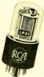
RCA-1P21. Current amplification is 2,000,000. Has S-4 spectral response. Maximum response at 4200 Angstroms. The tube has extremely low dark current.
