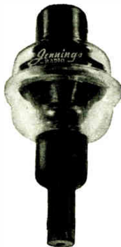
TYPE U—VACUUM VARIABLE CAPACITOR 10,000 Peak Volts Length 11\frac{1}{4}'' , Diameter 4\frac{3}{8}'' 250 to 350 mmfd. max.
