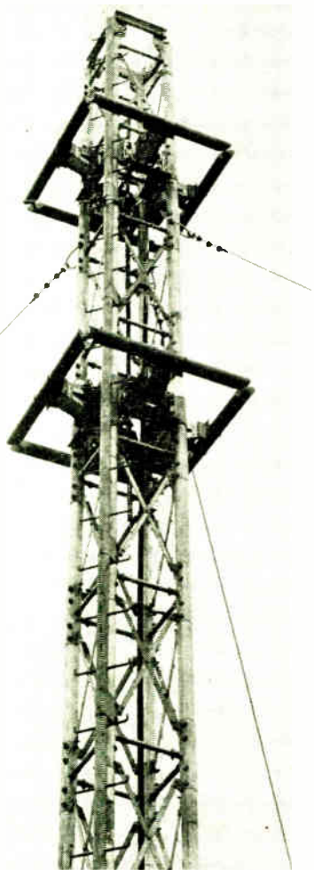
Two vertically stacked coaxial square loops designed for new 88-108 mc FM frequency
