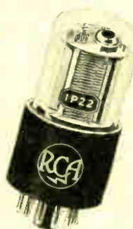
RCA-1P22. Current amplification is 200,000. Has S-8 spectral response. Maximum response at 4200 Angstroms. Range, approximately 3000 to 7500 Angstroms.
