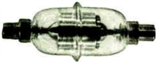
TYPE X—PEANUT , 5-25 mmfd., 17,000 Peak Volts, 20 Amps. Length 3\frac{1}{4}'' \pm 1/16'' , Diameter 1\frac{1}{4}'' \pm 1/16''
