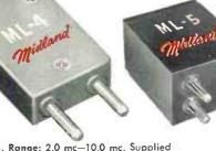
Type ML-4. Range: 2.0 mc-10.0 mc. Supplied per mil Type CR-5, CR:6, CR-8, CR-10 when specified. Holder is phenalic, gasket sealed. Pin diameter: .093 ± .002 Pin length: .400 ± .030
