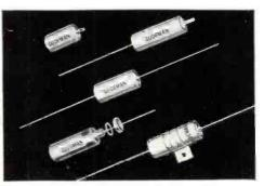
"XC" Plastic Film Dielectric Capacitors The development of the Gudeman "XC" capacitors provides high temperature capacitors that have exceptionally high insulation resistance, low power factor and low dielectric absorption. No voltage derating is required when used within a temperature range from  $-65^{\circ}$ C to  $+165^{\circ}$ C. Bathtub and rectangular case styles also are available.
