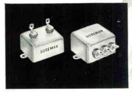
Bathtub Type Military Capacitors MIL-C-25 Types CP53, CP54, CP55 Case Styles Temperature Ranges: -55°C to +85°C -55°C to +125°C
