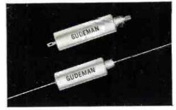
Miniature Feed-Through Capacitors The Gudeman Feed-Thru Capacitor, Types 271 and 272 is a three-terminal component designed to be used for R. F. Interference suppression in a manner similar to a low pass filter. The typical insertion loss characteristics for these Feed-Thru Capacitors when measured in a 50 ohm line are in accordance with MIL-Standard 220.
