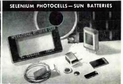
Self-generating photocells available in standard or custom sizes, mounted or unmounted. Optimum load resistance range: 10 to 10,000 ohms. Output from .2 MA to 60 MA in ave. sunlight. Ambient temperature range: -65°C to +100°C. Bulletin PC 649
