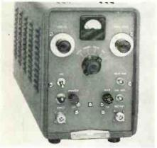
and constant output. Instruments are compact, and simple to operate. Model 492A covers 4 to 8 KMC with 30 db gain, 10 mw output and 15 millimicrosecond rise time. Model 494A cover 7 to 12.4 KMC with 25 db gain, 5 mw output, 15 millimicrosecond rise time. Both amplifiers can be used for wide dynamic range antenna tests and SWR measurements. Hewlett-Packard Company, 275 Page Mill Rd., Palo Alto, Calif. TELE-TECH & ELECTRONIC INDUSTRIES (Ask for 4-14)
