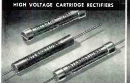
Designed for long life and reliability in Half-Wave, Voltage Doubler, Bridge, Center-Tap Circuits, and 3-Phase Circuit Types. Phenolic Cartridge and Hermetically Sealed types available. Operating temperature range: -65°C to +100°C. Specify Bulletin H-2
