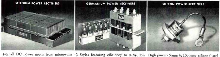
For all DC power needs from microwatts to kilowatts. Features: long life; compact, light weight and low initial cost. Ratings: to 250 KW, 50 ma to 2,300 amperes and up. 6 volts to 30,000 volts and up. Efficiency to 87%. Power factor to 95%. Bulletin C-349
