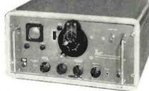
each of which usually has a more restricted frequency range. Unlike other heterodyne frequency meters, Type 504 is simple to use. Both CRT and aural presentation are available as well as a new exclusive interpolating dial which saves time and avoids ambiguity. Lightweight, therefore advantageous for field testing of transmitters, receivers and signal generators. Will deliver a signal of precisely known frequency at the RF input connector when used as a calibrating instrument.
