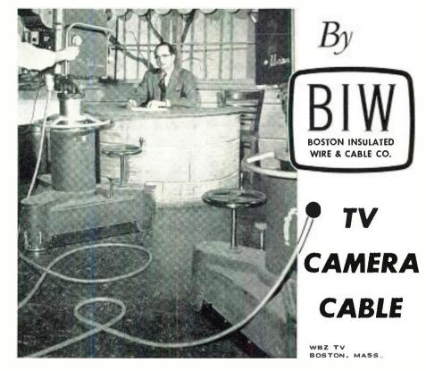
**LEADING STATION ENGINEERS** use BIW cables because they are so very flexible and smooth operating. TV camera engineers have chosen these cables for several reasons. The small diameter means less bulk in use, transportation and storage. The rugged Neoprene and Teflon construction resists mechanical damage and abrasion to an unusual degree.
