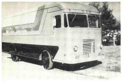
Air-conditioned 28 ft. truck houses two live color camera chains and associated equipment. Complete facilities are provided for on-air and closed-circuit applications, and for use at the studio location as a temporary color facility
