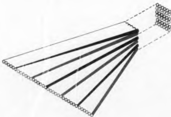
Fig. 14a: A line-to-raster transducer using fiber optics.
