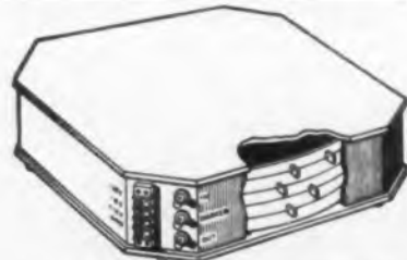
This cutaway sketch of the new digital function generator shows the mounting of the permanent magnets along the delay wire to provide for the desired pulse pattern.
