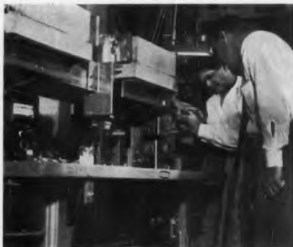
Fig. 3: Four formulations of silico-ceramic compounds are specially made for the coating of magnet wire with this piece of machinery.
