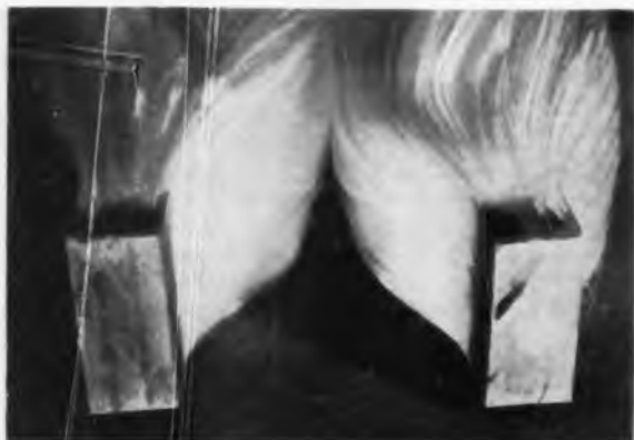
Fig. 9: Typical fiber bundle before surfaces are finished. (Photo courtesy of American Optical Co.)
