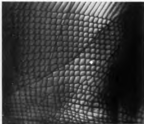
Crystal structure of bismuth telluride makes it especially suitable for the study of dislocations found in thin foils.
