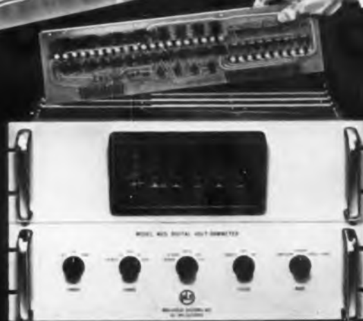
Digital voltmeters — Originated by NLS — permit rapid and accurate voltage measurements. New Series 20 unit — with one plug-in decade board removed — shows the use of Allen-Bradley fixed resistors.
