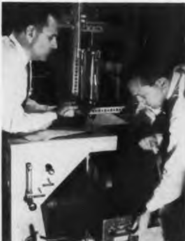
E. C. Spencer (left) and R. C. LeCraw of Bell Telephone Laboratories operate apparatus used to measure ferromagnetic resonance of yttrium iron garnet (YIG) samples. They have found that YIG has a much sharper resonance peak than any other ferromagnetic material, a property that will make it useful for a number of microwave applications.
