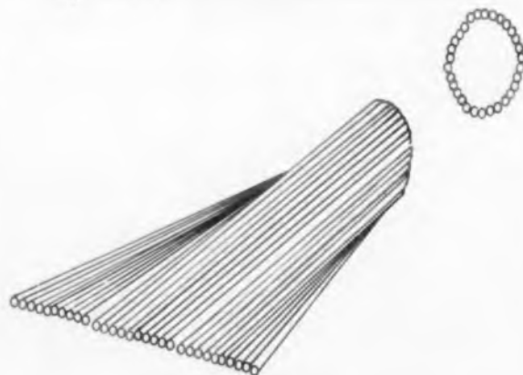
Fig. 14b: Line-to-circle transducer can be used for facsimile.
