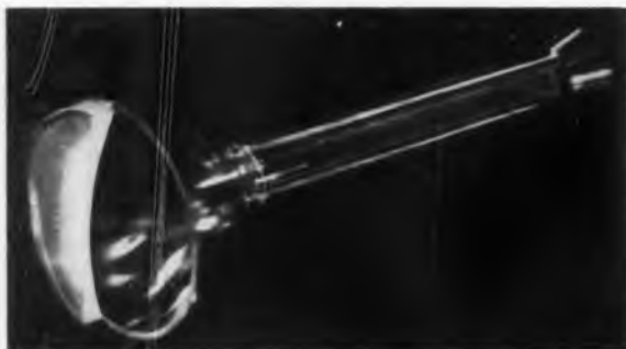
Fig. 10: Cut-away of a CRT with a fiber optic face-plate. (Photo courtesy Moog, Inc.)
