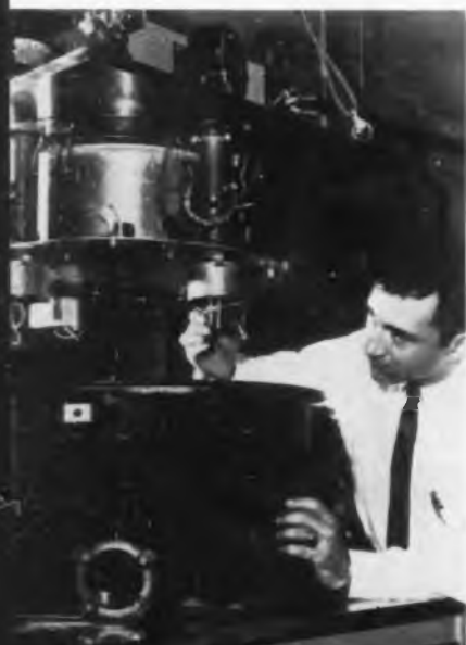
Researcher at GE's Schenectady, N. Y., lab prepares to test silicone grease in vacuum chamber that simulates space conditions.
