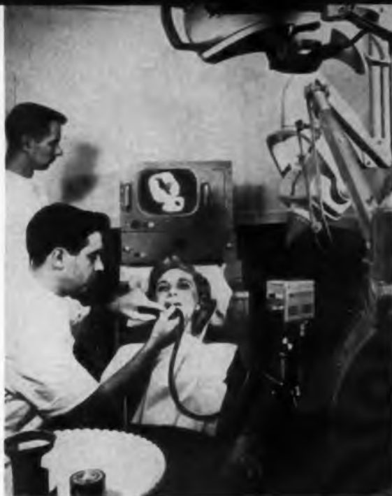
Fig. 13: Fiberscope is coupled to a closed-circuit TV so that observers have a good view of the patient's teeth. (Photo courtesy of AVCO)
