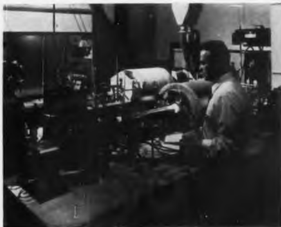
This diffusion apparatus is used to introduce controlled amounts of impurities into semiconductors such as silicon or germanium. Vapor pressure of these impurities is regulated by insertion into one of the furnace temperature zones. Diffusion depths and impurity concentrations are determined largely by the temperatures.
