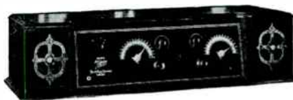
Super-Zenith VII (Not regenerative)—6 tubes—2 stages tuned frequency amplification—detector and 3 stages audio frequency amplification. Installed in a beautifully finished cabinet of solid mahogany—44½ inches long, 16½ inches wide, 10½ inches high. Door panels inlaid. Slanting panel of sheet bronze, mahogany finish, with scales and indicators in metallic relief. Gold plated pointers, to prevent tarnish. Compartments at either end for dry batteries. Can be operated on either wet or dry batteries. Either inside or outside antenna. Price (exclusive of tubes and batteries) $230
