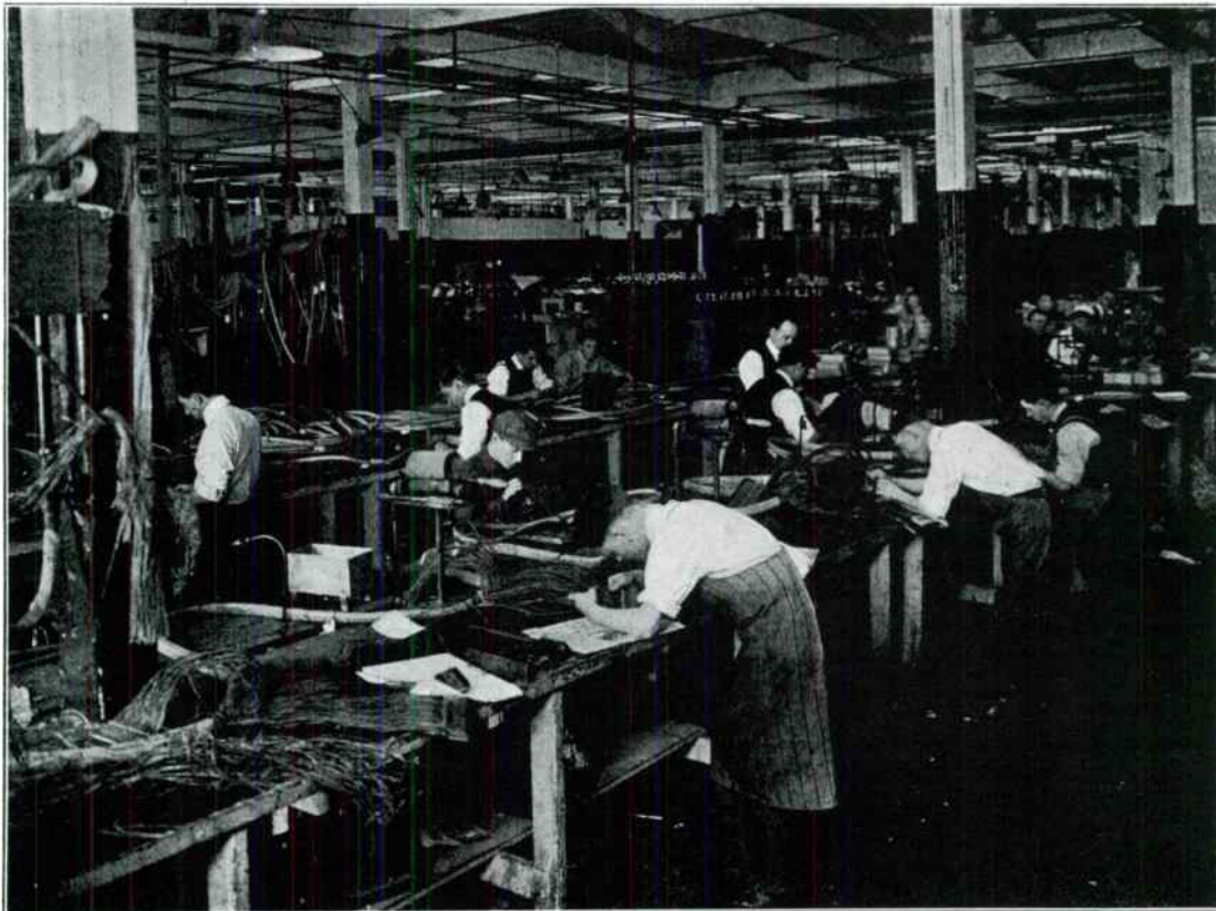
Wiring multiple jacks in the switchboard department.
