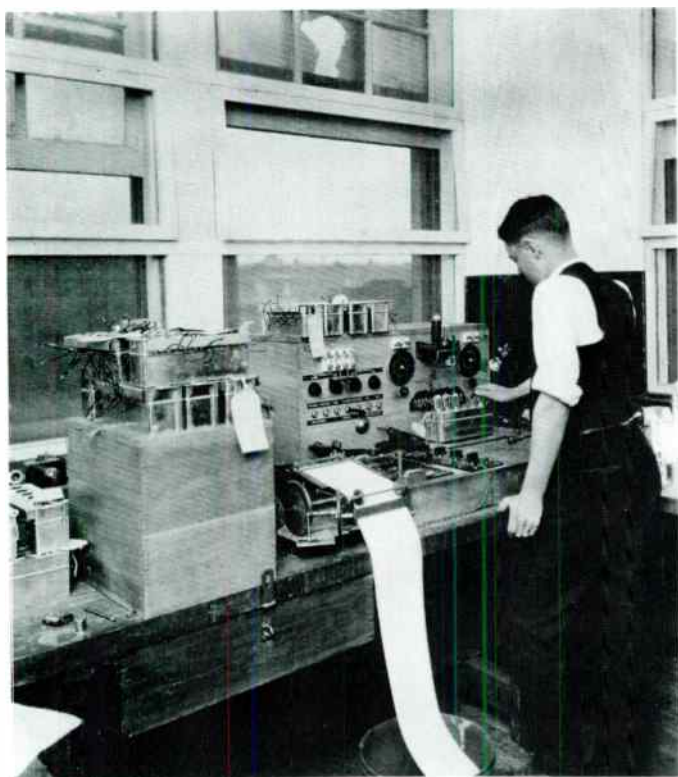
422608 TESTING BENCH FOR CATACOMBS OF RADIOLA SUPER HETERODYNE AND RADIOLA SUPER VIII. INDEX 654 7 1 24
