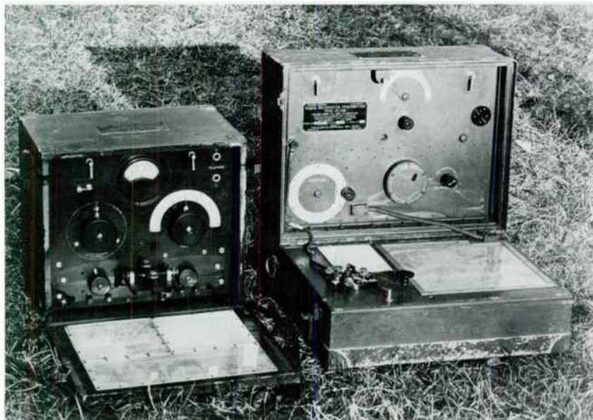
Later model (1929) BC-9 and the BC-148 that superseded it in 1935. Not shown: the one-turn loop antennas that attach to the backs of the sets.
