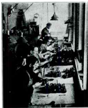
A faulty variable condenser means faulty performance. These men are inspecting every variable condenser used in Thompson Neutrodynes for mechanical defects.
