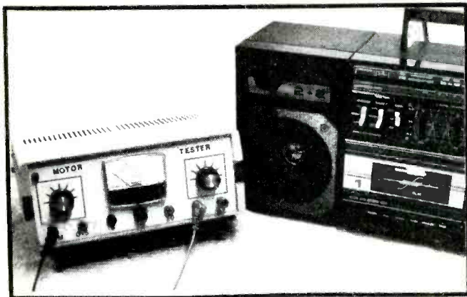
Figure 2: Dress up that front panel and make it look professional with decals, rub-on letters and numbers. Here the test instrument case has a plastic body with satin finish metal front panel.
