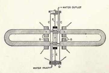
FIGURE 139—Cross section of Dubilier high current telephone relay.
