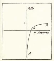
FIGURE 175—Grid potential-plate current characteristic of a pliodynatron.
