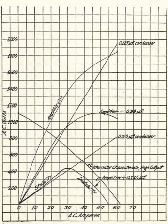
Figure 198—Effect of series condenser on stability of magnetic amplifier.
