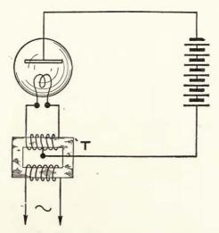
FIGURE 75—General Electric Company-White method of plate circuit connection.
