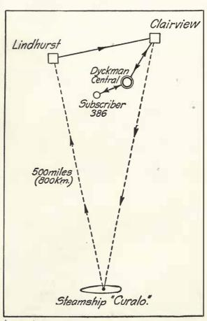
Figure 225—Typical ship-to-shore radiophone system.
