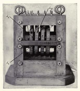
FIGURE 193—General Electric Company-Alexanderson "magnetic amplifier" radiophone control.
