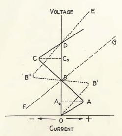
FIGURE 97—Dynatron voltage amplifier characteristics.
