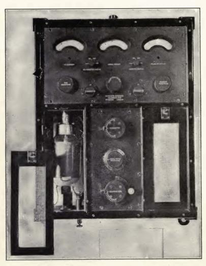
FIGURE 156-Marconi Company Sustained Wave Bulb Transmitter.
