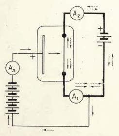
FIGURE 74—Illustrating Combined Lighting and Thermionic Currents.
