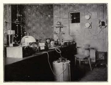
FIGURE 36-Ruhmer's radiophone transmitter.
