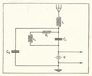
FIGURE 11—Fuller's method of increasing arc efficiency.
