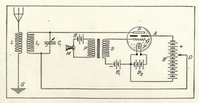
Figure 176—General Electric Company-Hull pliodynatron radiophone transmitter.
