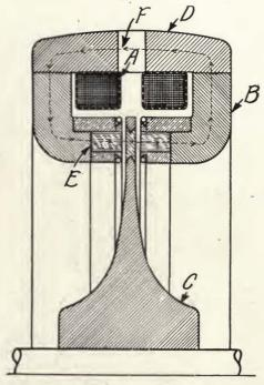
Figure 114—General Electric Company—Alexanderson alternator.
