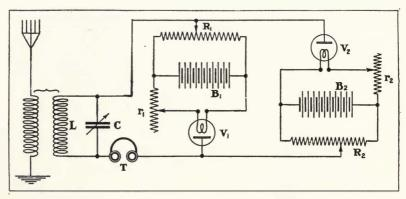
FIGURE 215-Marconi Company-Round balanced valve receiver.
