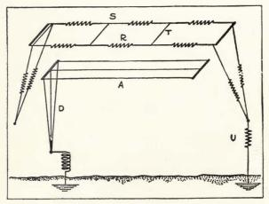
FIGURE 217—Dieckmann shielding cage for stray reduction.
