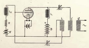
Figure 93—Western Electric Company—Colpitts oscillating circuit.
