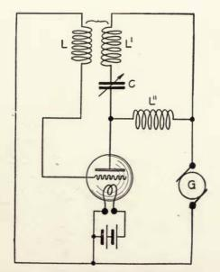
Figure 82—Arco-Meissner oscillating circuit.
