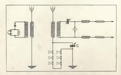
FIGURE 14-Poulsen radiophone transmitter and receiver.
