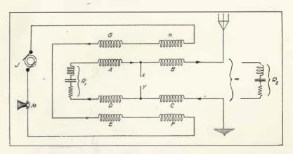
FIGURE 223—Fessenden duplex system for radio telephony.
