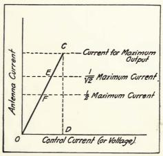
FIGURE 126—Complete linear modulation control curve.
