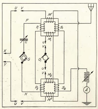
FIGURE 186—Telefunken Company-Kühn radiophone transmitter, 1913.
