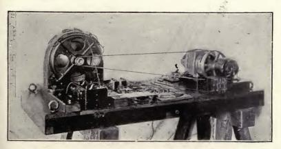
FIGURE 123—Recent General Electric Company-Alexanderson alternator of "gyro" type.
