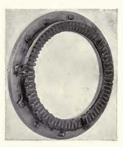
FIGURE 189—General Electric Company-Alexanderson telephone control relay; stator (field and armature).
