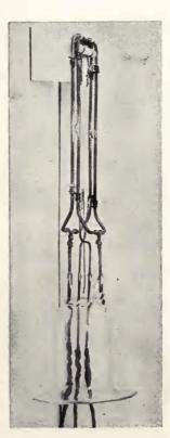
FIGURE 91—Filament and grid element of pliotron.
