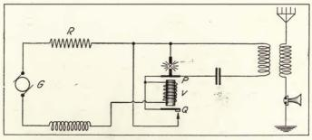
FIGURE 54-T. Y. K. radiophone transmitter.
