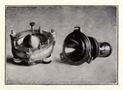
FIGURE 42—Interior of Scheller "multitone" gap.
