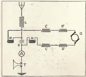
FIGURE 10-Typical arc radiophone transmitter.
