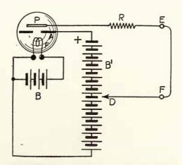
Figure 96—General Electric Company—Hull dynatron amplifier circuit.
