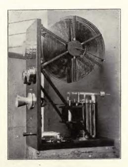
FIGURE 59—One-half kilowatt Hanscom radiophone transmitter.
