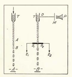
Figure 150—Essential parts of Majorana's liquid microphone.
