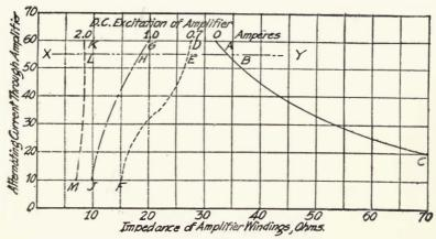
Figure 194—Characteristics of Alexanderson Magnetic Amplifier.
