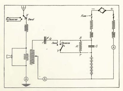
Figure 26—Telefunken series arc radio transmitter.
