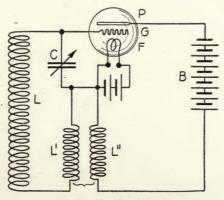
FIGURE 79—Oscillating circuit.
