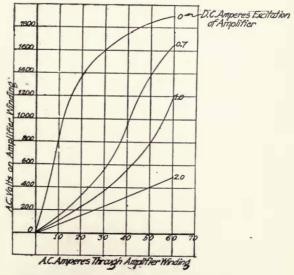
Figure 195—Characteristics of Alexanderson magnetic amplifier.
