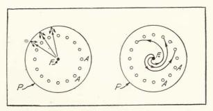
FIGURE 173—Effect of longitudinal magnetic field on electron paths in dynatron.
