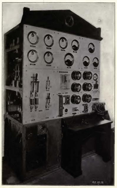
$\begin{tabular}{ll} Figure~187-Telefunken~Company~10~k.w.~alternator-frequency~doubler\\ radiophone~transmitter. \end{tabular}$
