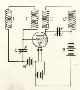
FIGURE 84—Marconi Company-Franklin Circuit, 1914.
