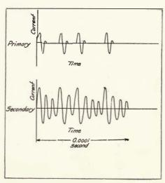
Figure 32—Irregular radio-frequent spark excitation of antenna.
