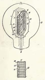
Figure 211—Western Electric Company-van der Bijl amplifier tube, 1915.
