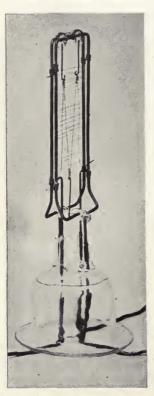
FIGURE 90—Filament and grid element of pliotron.
