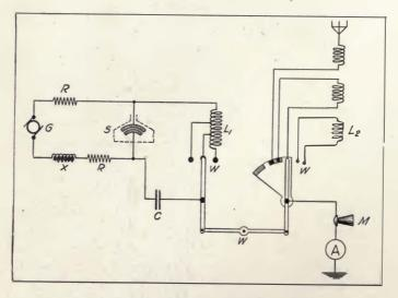
FIGURE 40—Lorenz Company radiophone transmitter.
