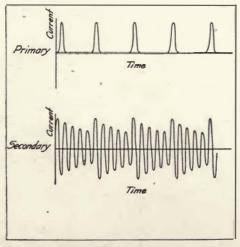
FIGURE 33—Regular radio-frequent impulse excitation of antenna.
