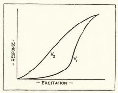
FIGURE 216—Valve characteristics with different auxiliary potentials.
