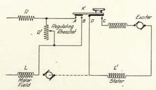
Figure 104—Goldschmidt alternator speed constancy system.
