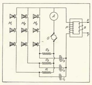
FIGURE 184—Telefunken Company-Kiihn system for utilising microphones in parallel on direct current.
