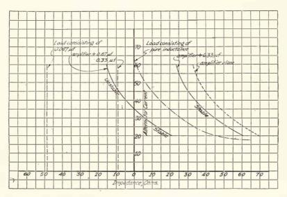
Figure 197—Effect of series condenser on stability of magnetic amplifier.
