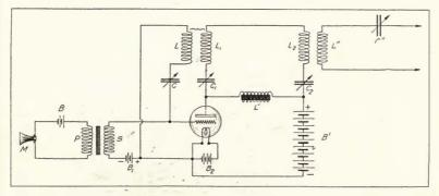
FIGURE 166—Western Electric Company-Colpitts modulation system, 1914.
