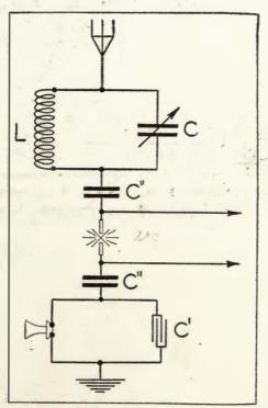
FIGURE 15—Fly-wheel Poulsen are circuit for radio telephony.
