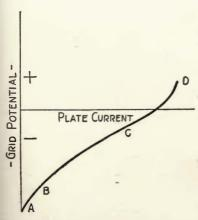
FIGURE 76—Relation between grid potential and plate current for pure electron amplifiers.
