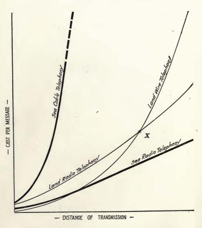
FIGURE 1—Comparison of cost; radio vs. wire telephony.
