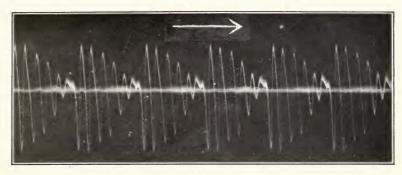
Figure 2-Oscillogram of vowel sounds "ah."
