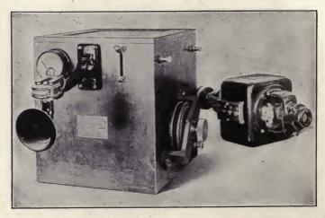
FIGURE 61—de Forest D. C. radiophone transmitter.
