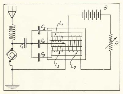
FIGURE 196—General Electric Company-Alexanderson magnetic amplifier, with series, short-circuiting, and shunt condensers.
