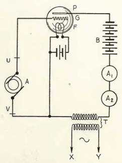
Figure 77—Amplification of alternating current energy.
