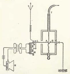
Figure 149—Vanni's liquid microphone relay.
