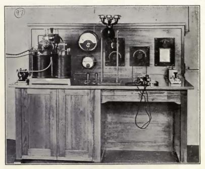
FIGURE 21—Berliner-Poulsen arc ship radiophone station.
