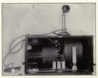
Figure 171—General Electric Company-White radiophone transmitter for direct current supply.
