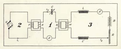
Figure 180—Control of radio frequency current in resonant circuit by variation of magnetisation of iron core of inductance.
