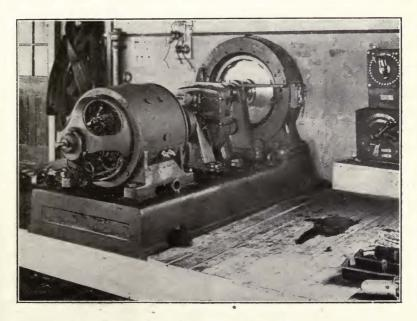
FIGURE 113—Telefunken Company 10 K. W., 10,000 cycle alternator.
