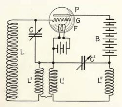
Figure 80—Plate circuit tuning in oscillating circuit.
