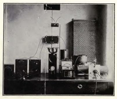
FIGURE 13-Danish Poulsen arc radiophone transmitter.
