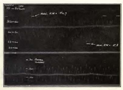
Figure 200—Oscillograms showing controlling telephone current and controlled antenna output of General Electric Company-Alexanderson 50 k.w. alternator and magnetic amplifier.
