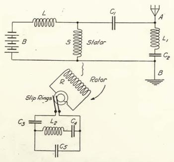
FIGURE 103-Winding of Goldschmidt alternator.
