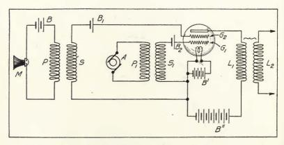
Figure 167—Western Electric Company-Heising modulation control system, 1915.
