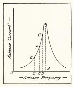
Figure 138—Detuning characteristic of radiophone transmitter.
