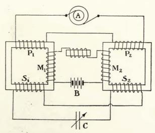
FIGURE 108—Telefunken Company frequency doubler.
