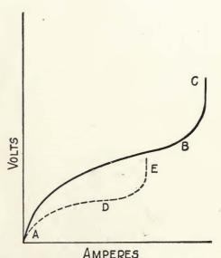
FIGURE 72—Relation between voltage and current for pure electron rectifier at a given temperature.
