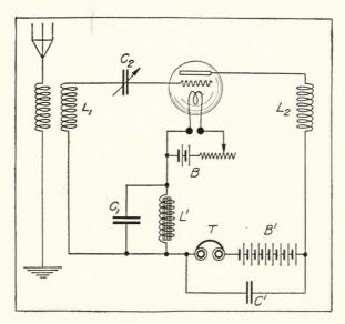
FIGURE 204—Armstrong regenerative circuit for radio frequency amplification.
