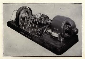
FIGURE 121-Intermediate type of Alexanderson alternator.
