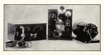
FIGURE 162—de Forest oscillion radiophone and radio telegraph transmitter and receiver (Type OJ3).
