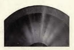
Figure 116—Portion of rotor of Alexanderson 100,000 cycle alternator, showing slots in disc.
