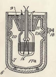
FIGURE 88—de Forest highpower tube construction.
