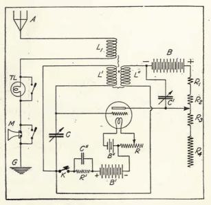
FIGURE 153-Marconi Company radiophone transmitter.
