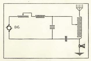
FIGURE 60—de Forest radiophone transmitter— D. C. type.
