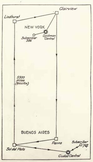
FIGURE 226—Typical duplex long distance radiophone system.
