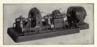
FIGURE 122—Recent type of 2 K.V.A., 100,000 cycle Alexanderson alternator.
