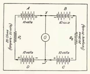
Figure 222—Principle of Fessenden duplex system.
