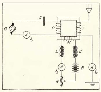
Figure 183—Telefunken Company-Kühn system of antenna current control.
