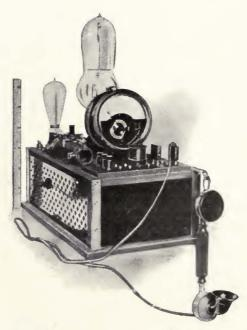
Figure 151—Telefunken Company-Meissner radiophone transmitter, 1913.
