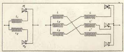
FIGURE 133-R. Goldschmidt's method of utilizing microphones in parallel.
