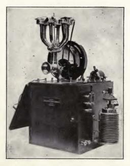
FIGURE 39—Complete Dubilier radiophone transmitter.
