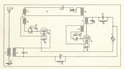
FIGURE 155-Marconi Company-Round radiophone transmitter of 1914.
