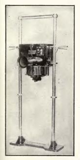
FIGURE 141—Heavy current Berliner microphone transmitter with fan cooling.
