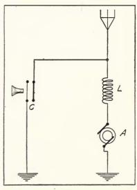
Figure 137—Fessenden condenser transmitter for radiophone work.
