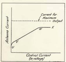
Figure 128—Typical incomplete nonlinear modulation control curve.
