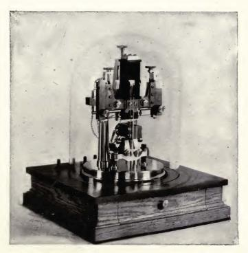
FIGURE 135—Fessenden heavy current telephone relay.
