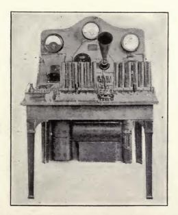
FIGURE 25—Telefunken Company series are radiophone transmitter.
