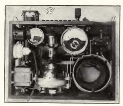
FIGURE 41—Lorenz Company aeroplane "multitone" transmitter.
