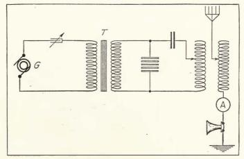
FIGURE 64—de Forest radiophone transmitter—A. C. type.
