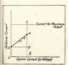
FIGURE 127—Incomplete linear modulation control curve.
