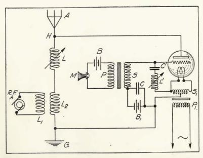
FIGURE 177—General Electric Company-Alexanderson-White alternatorpliotron radiophone transmitter.
