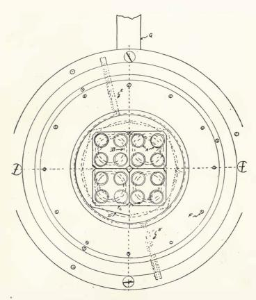
FIGURE 142—Front view of Egner-Holmström high current transmitter.
