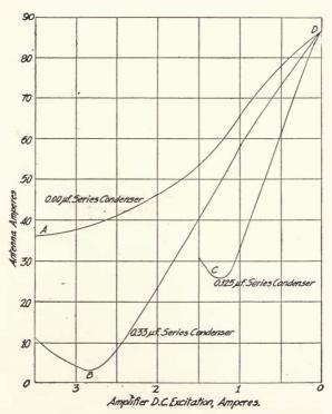
Figure 199—Control characteristics of magnetic amplifier.
