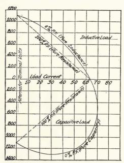
FIGURE 191—Load characteristics of 50 K. W., 50,000 cycle Alexanderson alternator.
