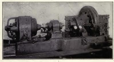
FIGURE 124—50 kilowatt, 50,000 cycle, General Electric Company-Alexanderson alternator.
