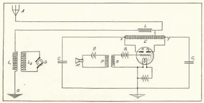
FIGURE 178—General Electric Company-Alexanderson alternator-pliotron control radiophone transmitter.
