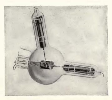
Figure 100—General Electric Company-Hull dynatron, showing internal structure.
