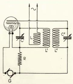
FIGURE 89—General Electric Company oscillating circuit.
