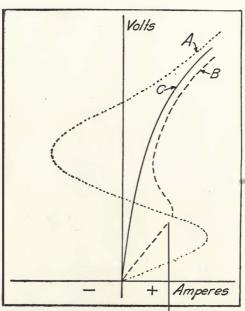
FIGURE 174—Characteristics of dynatron in various magnetic fields.
