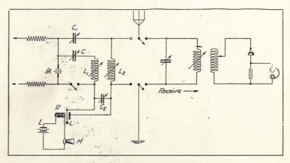
FIGURE 37-Dubilier radiophone transmitter and receiver.
