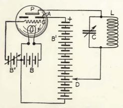
FIGURE 99—General Electric Company-Hull pliodynatron controlled oscillator.
