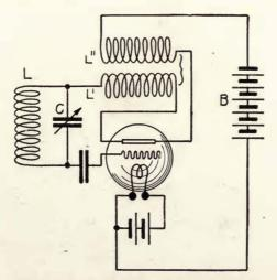
FIGURE 87—de Forest oscillating circuit, 1915.
