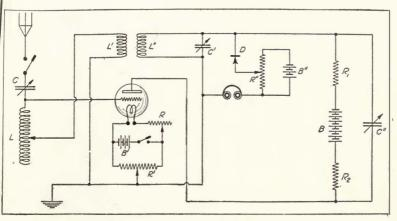
FIGURE 210-Marconi Company radiophone receiver.
