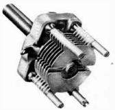
C804 — One gang. Ceramic insulation. Brass plates silver plated for RF efficiency. Available as model C801 for screwdriver adjustment. One hole panel mounting. Capacities 25PF, 50PF, 75PF, 100PF, 150PF.
