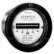
cycles, 50 cycles, 60 cycles, 400 cycles, 800 cycles and specials up to 1500 cycles; accuracy plus or minus 0.5 per cent. The individual reeds tuned to within plus or minus 0.3 per cent of their rated frequency; suitable for operation on 100-150 volts, 200-250 volts, 440 volts or low voltages. Trade name - "STANDCO", precision built, with reeds aged to prevent fatigue with resultant inaccuracies.
