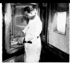
TEMPERATURE ALTITUDE CHAMBER has a 27 cu. ft. capacity. Tests from  $-100^{\circ}$ F. to  $300^{\circ}$ F., at altitudes from sea level to 100,000 ft.
