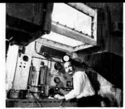
ICING WIND TUNNEL, with present 24 h.p. motors, has a maximum indicated airspeed in excess of 400 f.p.s. Work space cross section is 12x12 in.
