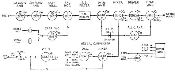
Fig. 1 - Block diagram of the HT-46 transmitter.
