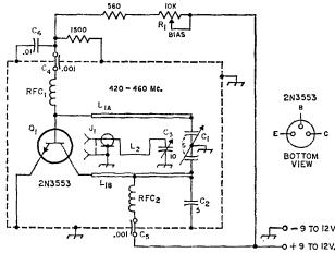
$L_1$ —3-inch parallel-conductor line of No. 10 bus wire (See Fig. 2).
