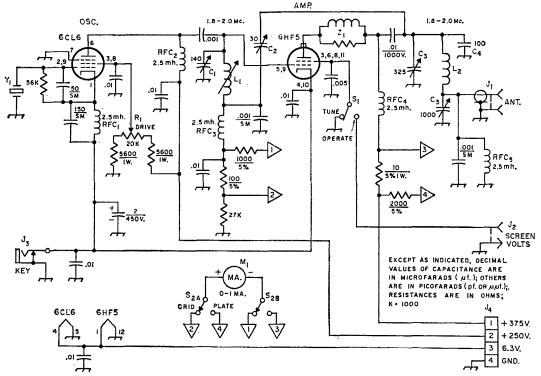
Fig. 1—Schematic diagram of the r.f. unit. Fixed resistors are  $\frac{1}{2}$ -watt composition unless otherwise noted. Capacitors are disk ceramic except those marked SM, which are silver mica. Capacitors bearing polarity marking are electrolytic and are in  $\mu$ f.
