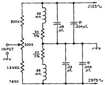
Fig. 4—The Mainline 7850 filter using 88-mh. toroids. The 0.004-µf. capacitor values (marked \*) are approximate. Short out the resistors in series with the toroids for maximum sharpness while tuning to frequencies shown. This filter is primarily for limiterless reception of 850 shift. The filters are each about 85 cycles bandwidth.
