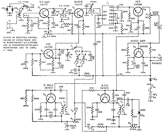
Fig. 1 — Circuit of the solid-state receiver. Capacitors are disk ceramic except those bearing polarity marking, which are electrolytic. SM = silver mica. Resistors are  $\frac{1}{2}$ -watt composition type. Terminal 11 has been added to  $Z_1$  as shown in Fig. 2. All unmarked capacitors associated with  $T_1$ ,  $T_2$ , and  $T_3$ , are contained inside the transformers and are supplied with them.
