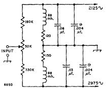
Fig. 3—The Mainline 8850 filter using 88-mh. toroids. Short out the resistors in series with the toroids for maximum sharpness while tuning to frequency. The 0.004-μf. capacitor values (marked \*) are approximate because of capacitance tolerance variation. The 8850 is for general reception; filters are each about 300 cycles bandwidth. Resistors are 5 per cent.
