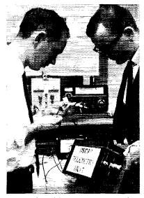
Bob Vogel, WØUBD (I.) and Jim Froemke, KØMHC, are shown examining thermisters for the Oscar Pulse Code Modulator telemetry unit at the IBM Development Lab. in Rochester, Minn. The 7-channel unit contains 150 transistors and 350 diodes. Future plans are to make use of integrated circuits to reduce the present  $5 \times 7 \times 12$ -inch size.
