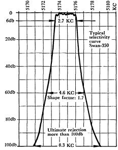
signals, especially the guy down the street with the big linear. In this respect, the Swan filter is superior to others being used in amateur sideband gear.
