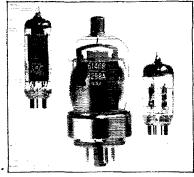
And no wonder. Power and receiving tubes alike used in any type of vehicle have to withstand high impact shock, almost continuous vibration, wide variations in temperature and humidity, frequent on/off cycling and even abnormal variations in operating voltages. Conventional tubes aren't necessarily designed to meet these conditions.
