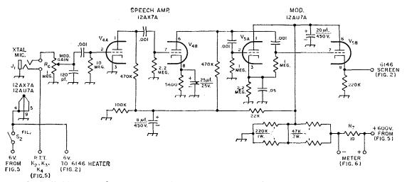
Fig. 3—Modulator circuit. Capacitances are in  $\mu$ f., and resistances are in ohms (K = 1000) unless indicated otherwise. Capacitors are disk ceramic or Mylar, except where polarization indicates electrolytic. Fixed resistors are  $\frac{1}{2}$ -watt unless indicated otherwise.
