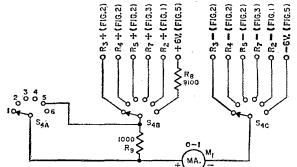
Fig. 6—Meter connections. M<sub>1</sub> is a 0-1-ma. d.c. meter, approximately 50 ohms resistance. R<sub>8</sub> and R<sub>9</sub> (resistances in ohms) are 5-percent resistors. S<sub>4</sub> is a 3-pole, 6-position rotary switch (Mallory 32361).
