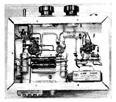
Fig. 5-Under-chassis view of the modulator assembly. The 12AX7 is at the right, the 6C4 is at the center, and the 6CM6 is at the left. Shielded wire is used for the filament circuit.
