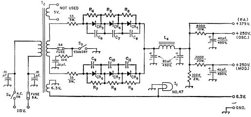
Fig. 6—Power-supply schematic. Capacitors are disk ceramic except those bearing polarity marking, which are electrolytic. Resistors are ½-watt composition unless otherwise indicated. Resistance is in ohms. K = 1000.
