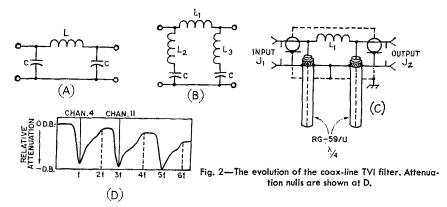
11. To effect a proper match to 73-ohm transmission line, quarter-wavelength transformers, made from sections of RG-54/AU, were used at each end of the filter. If 52-ohm feed line is to be used, coaxial connectors could be mounted at the input and output ends of the box and direct connection to the filter could be made with 52-ohm transmission line.
