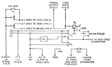
Fig. 5—Power-control circuitry.
