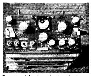
The converter and v.f.o. tuning controls are to the left and right, respectively, of the meter. Along the bottom of the panel are heater switches and the microphone jack to the left, meter switch at center, and controls for final-amplifier tuning, driver tuning, and antenna loading. Gain controls for the converter r.f. stage and speech amplifier are in the upper corners, left and right, respectively. The metal pieces at each end of the panel are lamp shields.
