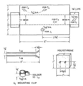
Fig. 2—Layout for the copper trough, the tuned line, and the polystyrene insulating block. Hole diameter for C<sub>4</sub> and C<sub>5</sub> is dependent upon type of feedthrough capacitor used.
