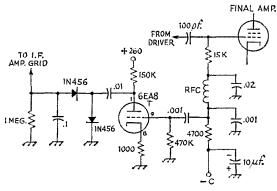
Fig. 3—The amplified a.l.c. circuit used in the HT-46. Capacitances are in  $\mu$ f. except as indicated. Resistors are  $V_2$  watt. The 4700-ohm resistor may be made larger or smaller to increase or decrease the d.c. output voltage from the rectifier; the value shown is used with the 6HF5 final amplifier in the HT-46.
