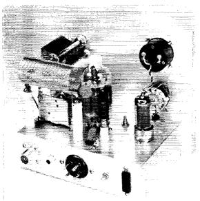
Fig. 2—Top-rear view of the r.f. assembly. Antenna connector is at left on chassis apron and next to phono connector for screen voltage input. Power receptacle is at center with ground post to the right. The 4-connector socket at the far right is not used and was installed for future experiments with v.f.o. operation.
