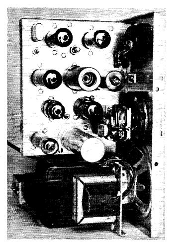
Vertical chassis mounting is used, with the chassis "top" on the left, as viewed from the front panel. A separate chassis is used for the power supply, at the bottom in this view.
