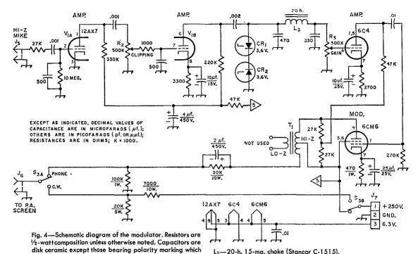
are electrolytic. CR<sub>1</sub>, CR<sub>2</sub>—3.6-volt Zener diodes. (1N747 or equivalent).
