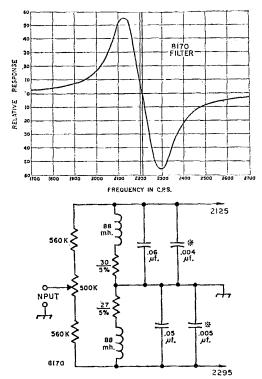
Fig. 5—The Mainline 8170 filter for 170 shift. Each filter is about 85 cycles wide using 88-mh. toroids. Capacitor values marked (\*) are approximate, and should be selected to tune the toroids to the indicated frequencies.
