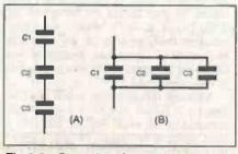
Fig.2.8. Capacitor in series (A), and parallel (B).
