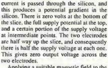
Applying a suitable magnetic field to the device "skews" the current flow and the potential gradient, producing an imbalance in the output potentials. The stronger the magnetic field, the greater the difference in the output voltages.
