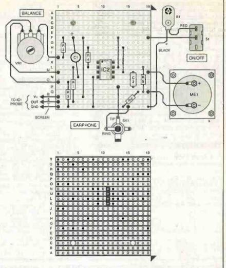
Fig.4. Stripboard component layout interwiring and details for breaks required in the underside copper tracks.
