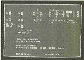
Photo 2.4. Interactive computer screen for calculating serial and parallel capacitor combinations.
