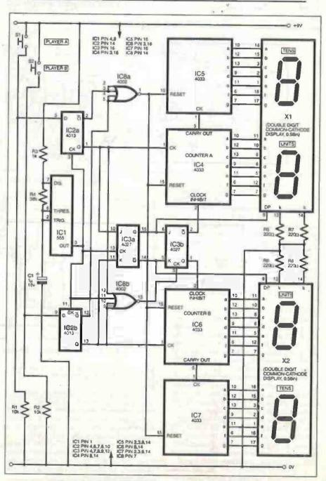
Fig.8. Circuit diagram for the Squash/Badminton Scorer.
