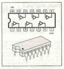
Fig.2.10. Pinouts and typical case style for 74HC04 hex inverter gate. Note the inversion gate symbols within the pinout drawing.
