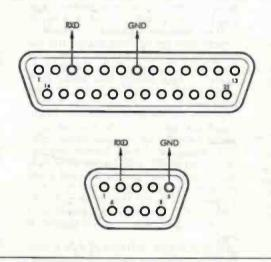
Fig.2. Interface connection details for 25-pin and 9-pin serial ports.
