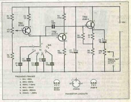
Fig.8. Circuit for a linear sawtooth generator.
