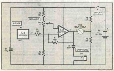
Fig.3. Complete circuit diagram for the Magnetic Field Detector.
