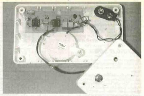
Positioning of components and circuit board inside the prototype case. Note the I.d.r. "window" hole and Reset switch position in the lid. The space to the right of the p.c.b. is for the battery holder.
