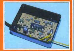
**MAGNETIC FIELD** DETECTOR **Investigate static** or a.c. fields
