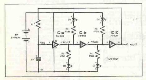
Fig.2.15. Circuit diagram for the oscillator experiment.
