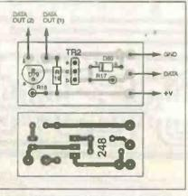
Fig.4. Printed circuit board details for the Serial Port converter.
