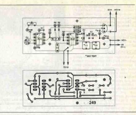
Fig.2. Printed circuit board component layout and full size copper foil master pattern.
