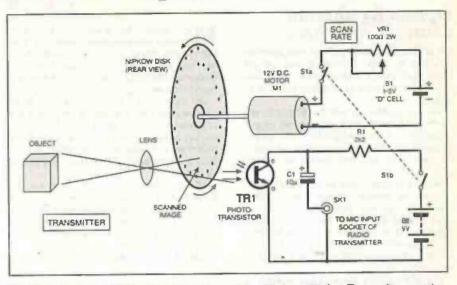
Fig. 7a. Circuit/mechanical arrangement of the Nipkow 25-line Transmitter section.
