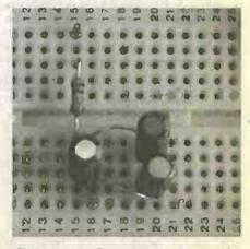
Photo 2.5. Breadboard layout for -examining capacitors in parallel.
