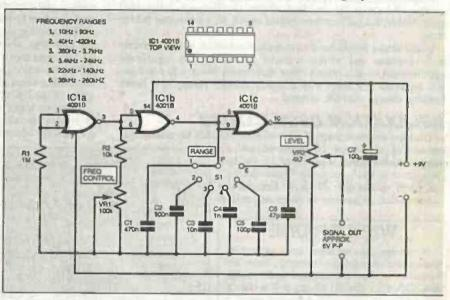
Fig.5. Circuit diagram for a wide range, square wave generator using a 4001B quad 2-input NOR gate I.c.
