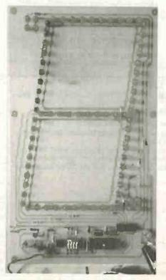
Completed "7-segment" Giant Display module. The figures measure 178mm by 100mm approx.
