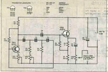
Fig.2. Circuit diagram for an adjustable spot frequency sinewave oscillator with an heavy negative feedback in order to stabilise sigoutput buffer stage.
