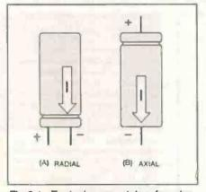
Fig.2.1. Typical case styles for electrolytic capacitors.
