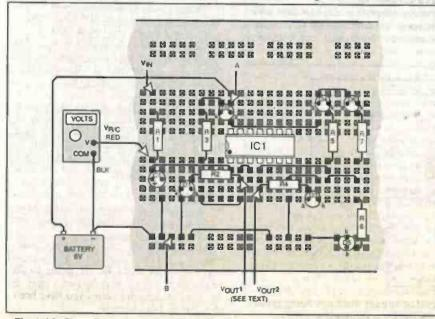
Fig.2.13. Breadboard assembly of Fig.2.11 modified to include five more I.e.d.s.
