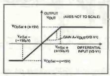
Fig.3. Graph showing the relationship between op.amp differential input voltage and its output voltage. Saturation occurs when any increases in the magnitude of the differential input do not result in further increases in output voltage. The values shown are an example for an op.amp with a gain of 100,000 and a maximum output voltage of ±15V. The gain of the op.amp is equal to the slope of the graph between the saturation points.
