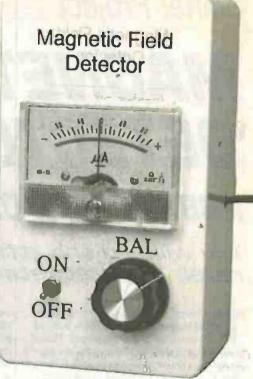
Magnetic Field Detector front panel layout, The Hall effect sensor is mounted externally in a probe arrangement, such as an old pen case, and connected to the circuit board via the screened cable.
