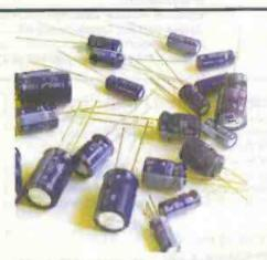
Photo 2.1. A selection of electrolytic capacitors (radial construction).
