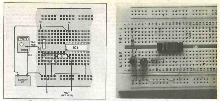
Fig.2.11 and Photo 2.6, breadboard layout for the first timing experiment using an inverter gate.
