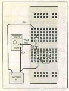
Fig.2.9. Breadboard layout for capacitors in parallel experiment.
