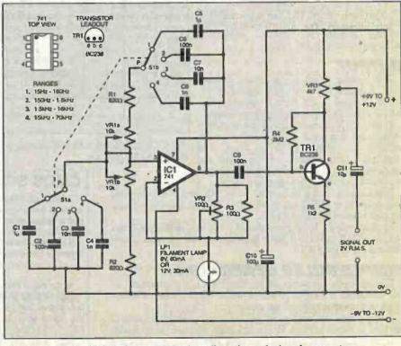
Fig.3. Circuit diagram for a low distortion a.f. signal generator.
