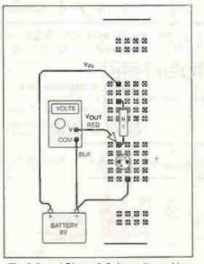
Fig.2.2 and Photo 2.2, breadboard layout for the first resistor/capacitor timing experiment.
