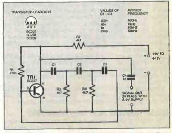
Fig.1. Circuit for a simple spot frequency sinewave oscillator.
