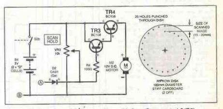
Fig. 7c. Improved Receiver add-on with Scan/Sync control (VR3).
