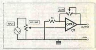
Fig.1. Circuit to illustrate the two types of volume control.
