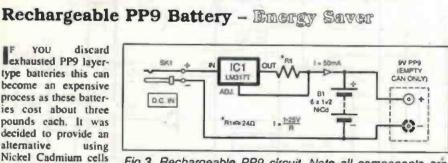
Fig.3. Rechargeable PP9 circuit. Note all components are housed inside the discarded PP9 casing.
