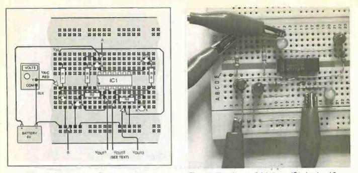
Fig.2.14 and Photo 2.7, layout for the oscillator experiment, (Fig.2.15). Note the new link between IC1 pins 4 and 5.
