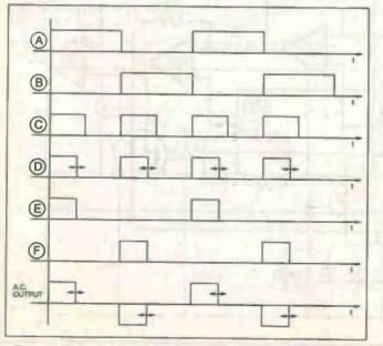
Fig. 11b. Output waveforms at various stages of the circuit.
