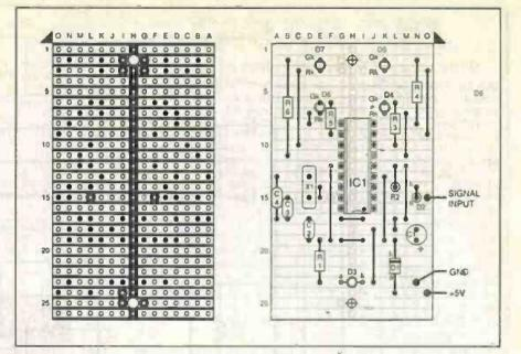
Fig.2. Component layout and stripboard track details for the PIC Micro-Probe.
