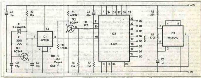
Fig.1. Circuit diagram for the Simple Serial Inferface add-on. It operates at 9600 baud.
