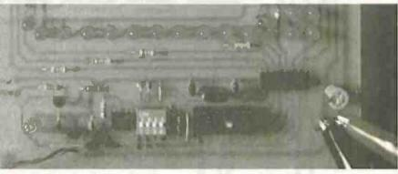
Completed control and power supply area of the Display p.c.b.
