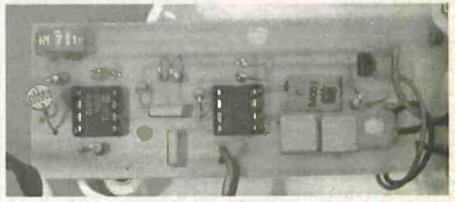
Components mounted on the completed circuit board. Note that a single cermet film resistor has been used for R7 (see text).
