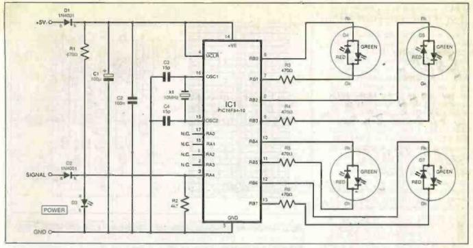
Fig.1. Complete circuit diagram for the PIC Micro-Probe,
