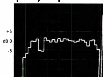
Fig 5 The third-octave frequency response is similar to the impulse response, except at low frequencies where it is more accurate and detailed. The cancellation suckout at 150Hz is clearly visible, plus output maintained down to 30Hz.
