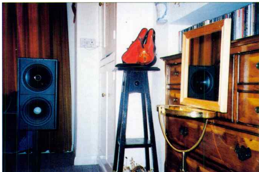
The mirror test: the mirror leaning against the chest of drawers shows an image of the loudspeaker. This identifies the position of an acoustic image - a source of reflections.
