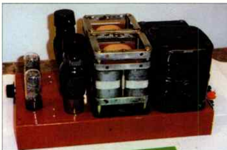
In the amplifier competition, 3rd prize went to Roy Marsh for this twin-807 single-ended design with home wound output transformers.
