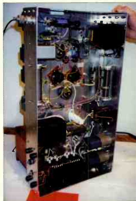
The underside of Chris Johns' amplifier houses numerous transformers, for D.C. heaters and such like, as well as dry capacitors, rheostats and many other parts not seen nowadays.
