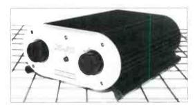
components, the X-A1 is a six-input line-level amplifier. Power output, claimed as 50watts into 80hms and 100watts into 40hms, has been maximised by locating the power supply outboard. PSU connection is via a Neutrik XLR socket.
