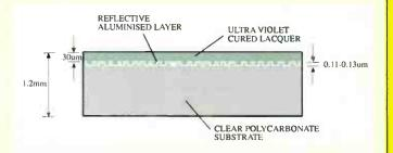
A slice through a CD shows how close to the disc's surface the aluminium layer is on the label side.
