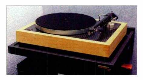
The modified Thorens TD150 uses the original platter, bearing and motor but everything else has been changed.
