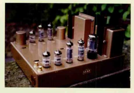
redesigned the range and added to it. There was the TL12+ with its EL84s, the TL25+ with the larger EL34s, and the most powerful of the three, the TL50+ which used a pair of KT88s. No prizes for guessing the output power of each! The sad thing is, the bigger they
