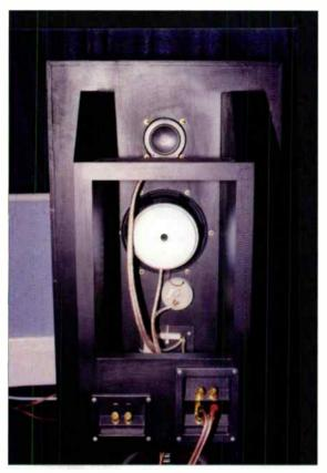
At the rear of the loudspeakers are two binding trays. The one on the left runs direct to the woofer while the one on the right feeds the tweeter/midrange passive crossover.
