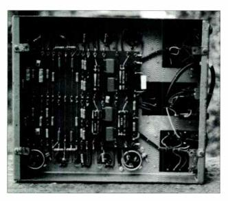
Unless your Stereo 20 is a mint original sample, the best bet is to rebuild it with modern components like Elna electrolytics and metallised-polypropylene coupling caps.
