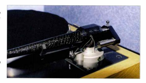
The cabling exits the arm at the pivot point on the prototype. This will be changed on production examples to reduce potential electrical interference.
