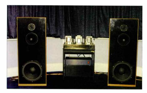
The open-baffle loudspeakers flank the equipment rack which contains, from top to bottom, the valve power amp, active crossover and MOSFET power amp.
