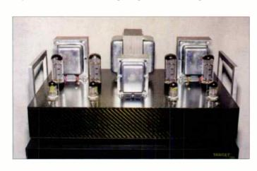
The valve amp's moulded carbon-fibre chassis has the large output and mains transformers bolted to its upper surface, along with the PSU inductor and valves.
