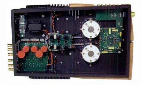
The input and driver stage to the right of the picture uses yellow 0.22uF 250V and 400V film and foil coupling capacitors. In the centre of the chassis are the multiple heater reservoir caps. The red caps at the rear of the chassis are for the High-Tension supply that feeds the 845 and ECC82 valves.
