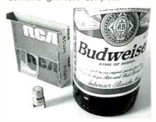
Around this time the Nuvistor appeared. It was almost as small as a transistor, supposedly more reliable and suitable for high-frequency work, unlike transistors of the time. The Nuvistor used one-third the heater power of a valve - 0.135A at 6.3V instead of 0.3A. RCA's 6CW4 Nuvistor pictured here was an RF triode designed for VHF communications. Its anode needed around 135V and dissipated just 1 watt.
