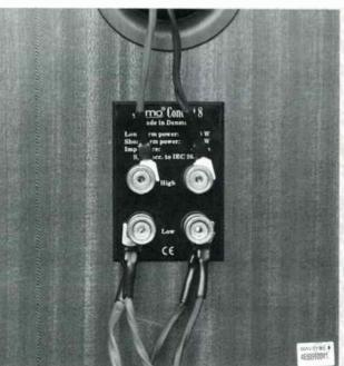
Doubling up loudspeaker cables, as shown here on the bass section of the Jamo a cheaper, more disposable point down to the stone surface Concert 8's crossover, reduces cable resistance and inductance by up to 50%. set of 'speakers first.
