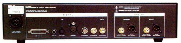
The thin, wide 1<sub>2</sub>S.enhanced input joins an impressive array of socketry on the Processor 3's back panel.
