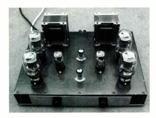
Chris's home-made push-pull amplifier is built from the ground up and uses KT66s in its output.
