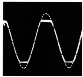
If you push an amplifier beyond its rated power output, it will start to 'clip' the signal. This can destroy loudspeaker drivers. The dotted lines show the unclipped waveform.
