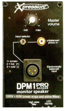
Most active loudspeakers possess potentiometers to adjust input level, as well as a choice of sockets (RCA and XLR in this case).
