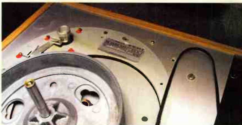
Above: speed change on the Thorens is achieved with a stepped pulley and guide lever. Below: The bearing on the TD160 (right) is slightly larger than the TD150's.
