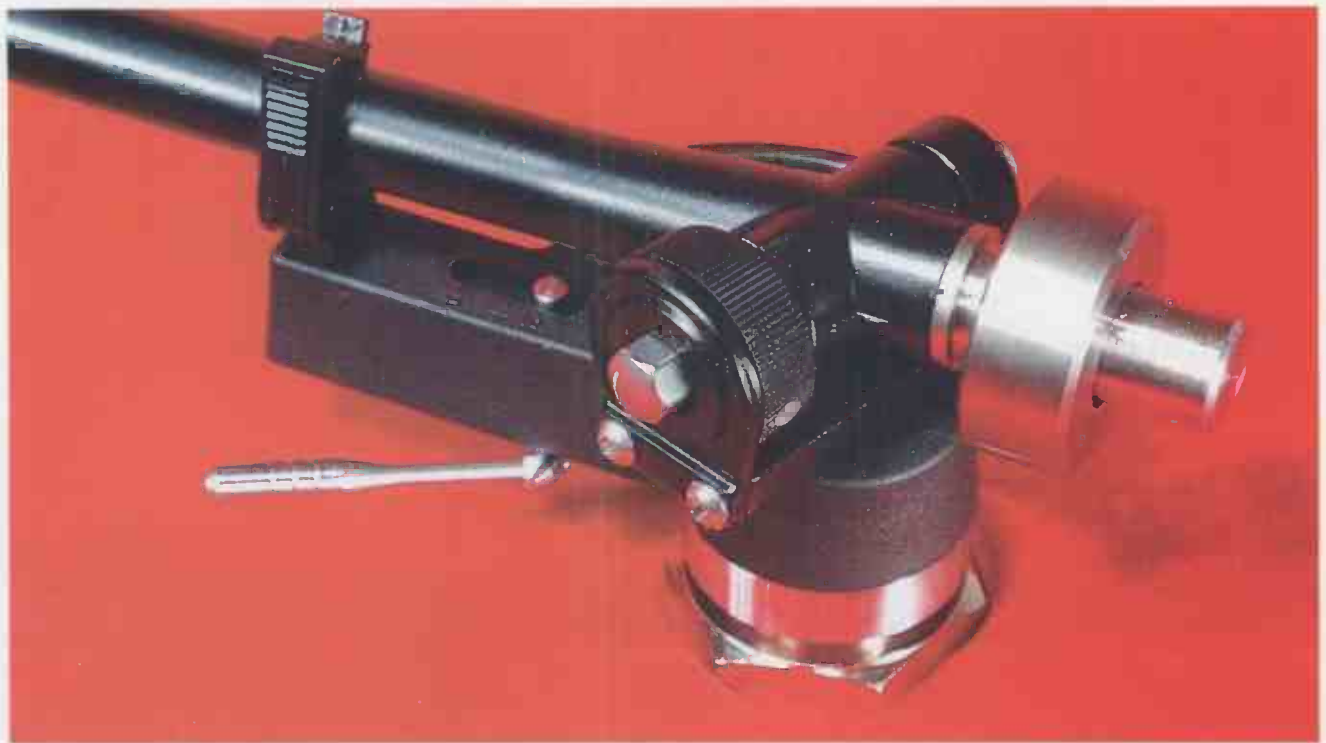
The unmodified RB300 has a screw-in rear stub along which slides the counterweight, decoupled by rubber rings.
