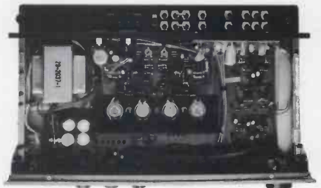
Inside NAD's 3020 amplifier, a classic second-hand integrated bargain.
