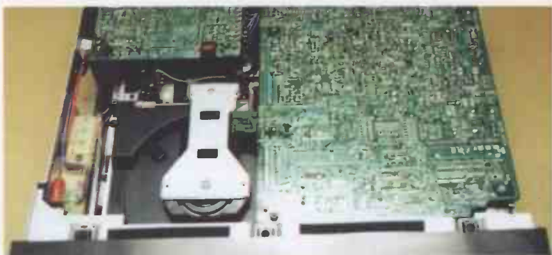
It's easy to gauge the CDP-101's vintage from the component density and complexity on the PCBs.
