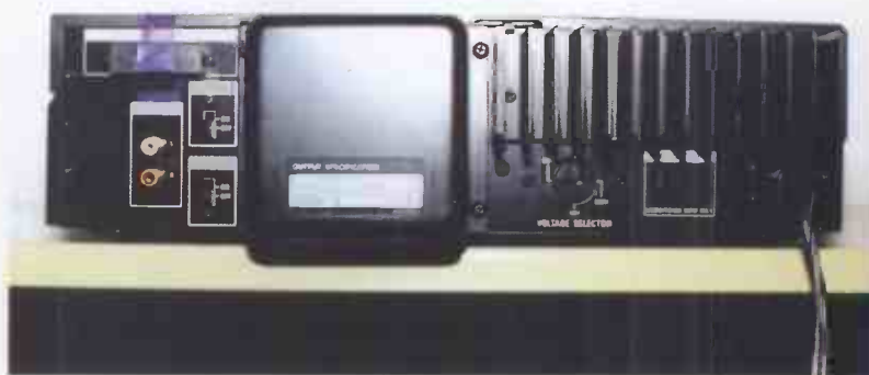
Many better-built older players (like the Pioneer PD-91) had chunky transformers on their back panels.
