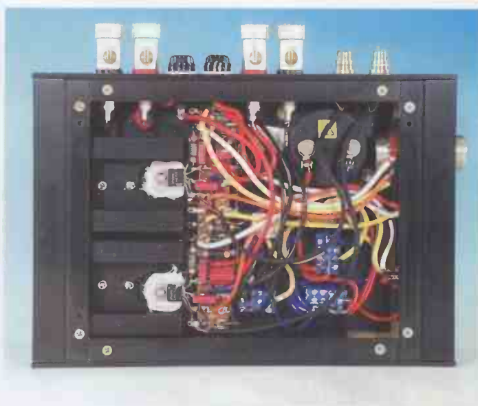
It might look like a bit of a rat's nest, but the Music-6's hardwiring boosts sound quality.
