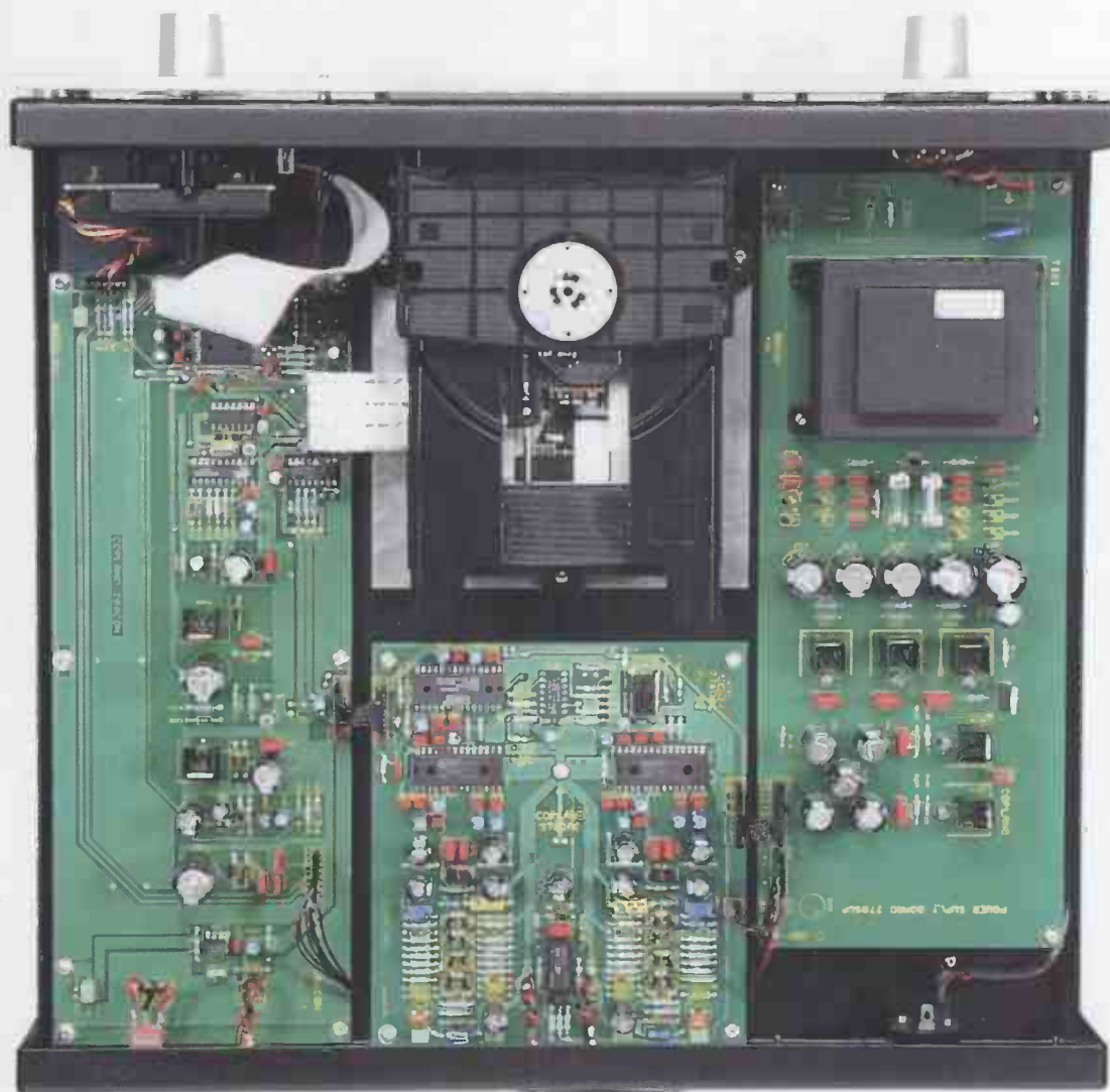
Unlike many CD players these days, the Copland draws its power from a single E/I core transformer.
