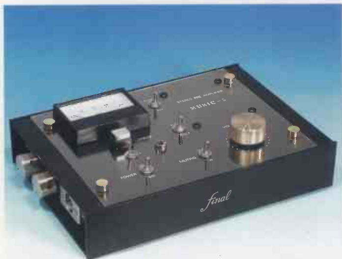
Both the pre and power are housed in classy aluminium extrusions with perspex top plates.
