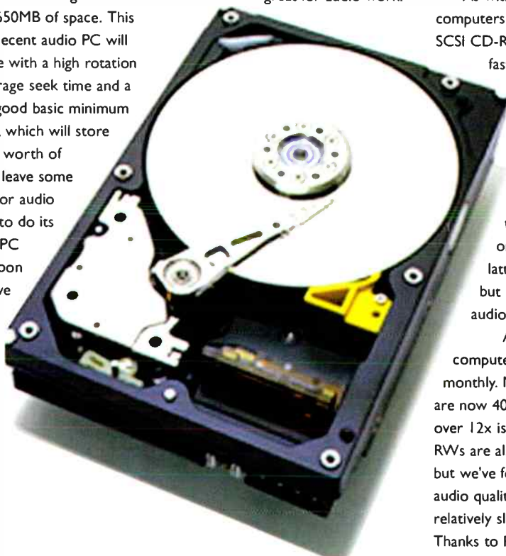
An IBM hard disc drive showing an internal sensor arm and multiple platters.
