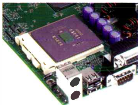
An AMD Athlon Socket A processor, sitting behind PS/2 and USB ports.
