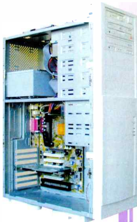
A full size tower case gives plenty of working space and will house a variety of audio drives.
