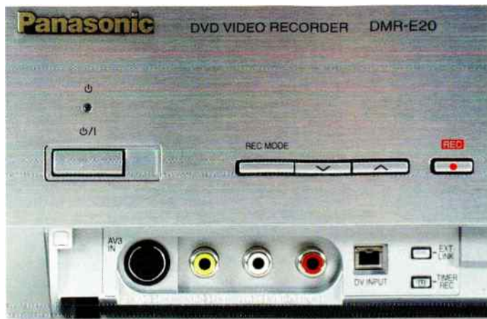
The front of the machine houses the analogue and S-Video sockets
