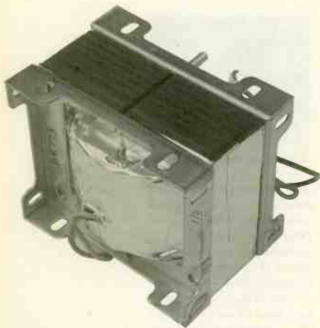
Fig.3 Finished transformer ready for refitting.
