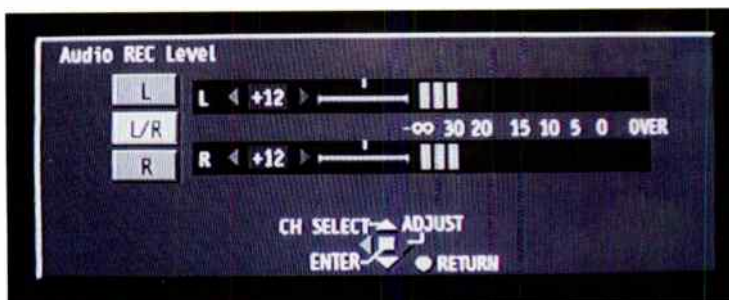
A simple recording level display appears on TV, allowing level and balance to be adjusted manually.
