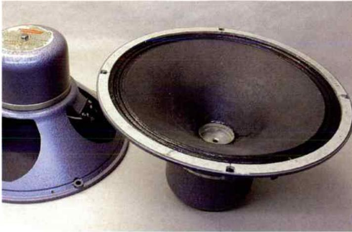
**Goodmans Axiom 150 dating from the late 1950s is typical of large bass drivers of its day (dust cap and whizzer cone removed in this example). These were ideally suited to large, aperiodic, cabinets and Goodmans marketed one of the first commercial aperiodic vents!**
