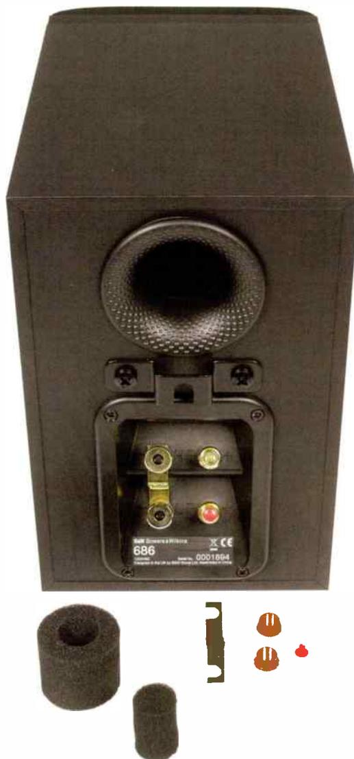
***B&W supply a two-part bung to tune bass output of their small 686 loudspeaker; insert bung for wall mounting. Leave it out for stand mounting. If you want to biwire, remove the links, as shown at right. Remove the small plastic plugs too when 4mm plugs are used...***
