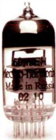
**Electro-Harmonix 6922 valve from Russia, a good starting point.**
