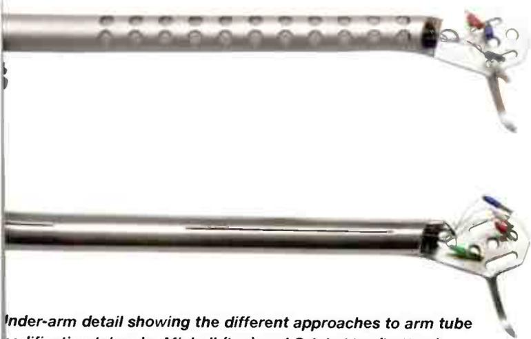
Under-arm detail showing the different approaches to arm tube modification taken by Michell (top) and Origin Live (bottom).
