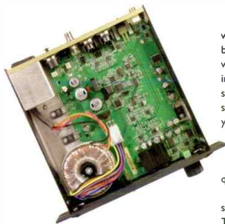
is driven directly from the reference crystal oscillator and feeds three NE5532 op-amps per channel.
