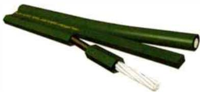
The 2 conductors each are made of 126 strands of high purity Matched Crystal OFC with a very dense pure silver coating. Each conductor exhibits a cross-section area of 2.53 mm<sup>2</sup>, closely approaching AWG 13.
