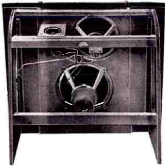
**Wharfedale SFB3 rear view. Note cutouts in side 'wings' to reduce resonance and bracing to improve stability. As expected the bass unit is positioned closer to the floor boundary and the midrange unit higher up. A cone treble unit, on its own baffle, points upwards at the rear!**
