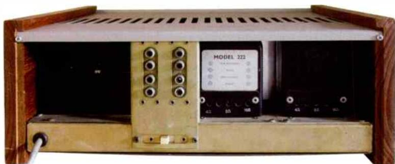
*Basic connections, with two pin speaker sockets.*
