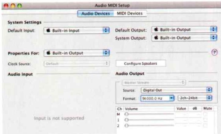
The 'Format' set is the Mini's output data rate, irrespective of the music file rate. A data rate of 96kHz, shown here, is the maximum. 'Digital out' means optical S/PDIF.
