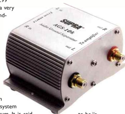
between any two line-level components in a hi-fi or home cinema system to avoid ground loop hum. It is said to be "a true high-end hi-fi design using toroidal transformers with wide frequency range and low distortion, even at the lowest frequencies". The chassis is made from extruded aluminium, which helps prevent any RFI pick-up. Quality gold-plated phono-sockets complete the picture. For more details, call +44(0)1223 441 299 or click on [www.supracables.co.uk](http://www.supracables.co.uk).
