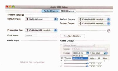
Sampling rate options for USB were 44.1 and 48kHz with our Intel Mac Mini running Leopard, connected to a Cambridge Audio DAC Magic able to process 96kHz.
