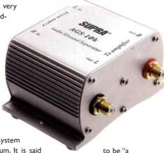
true high-end hi-fi design using toroidal transformers with wide frequency range and low distortion, even at the lowest frequencies". The chassis is made from extruded aluminium, which helps prevent any RFI pick-up. Quality goldplated phono-sockets compete the picture. For more details, call +44(0)1223 441 299 or click on www.supracables.co.uk.
