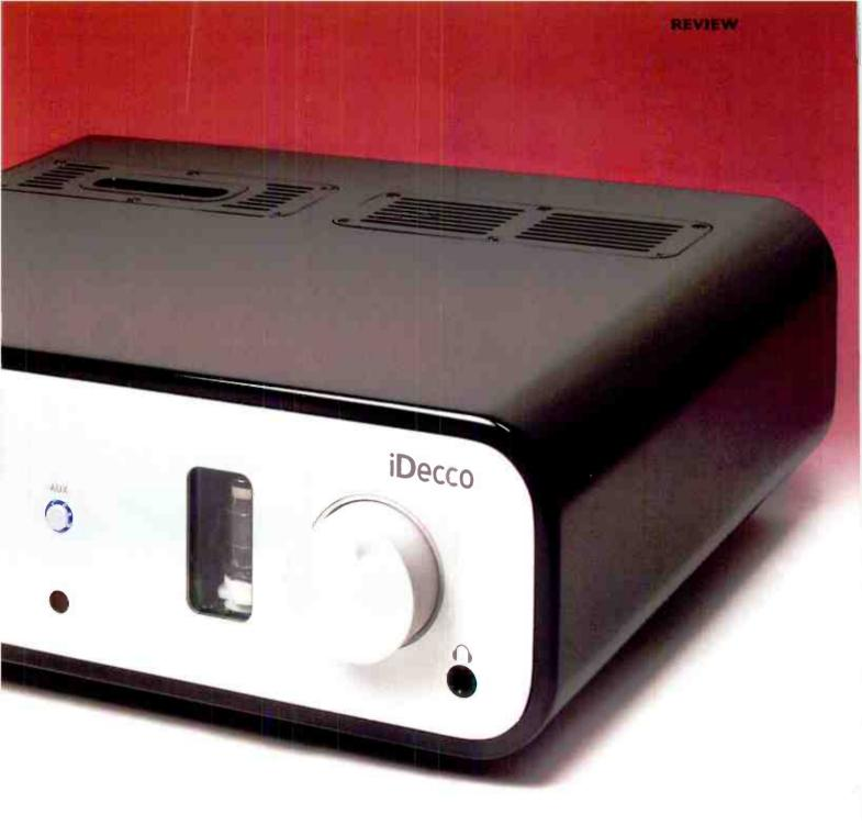
Its patented jitter reduction circuit reclocks the digital signal before passing it through a high-resolution 24/96 upsampling processor. Each digital input is transformer-coupled so noise associated with ground problems and switching power supplies from computers is said to be eliminated. The USB connection is galvanically isolated, eliminating noise generated by your computer's switching power supply and greatly improving sound quality, it's claimed.
