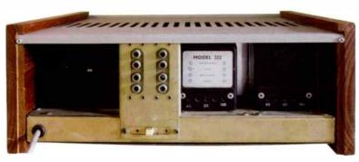
Basic connections, with two pin speaker sockets.
