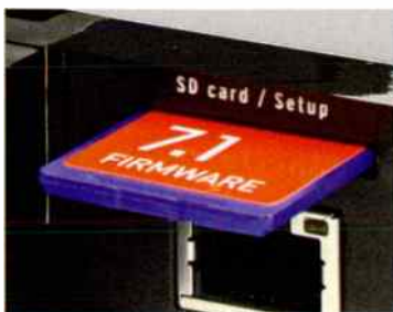
Configuration and software updates are loaded onto the Devialet 120 via an SD card which slots into the rear of the unit.
