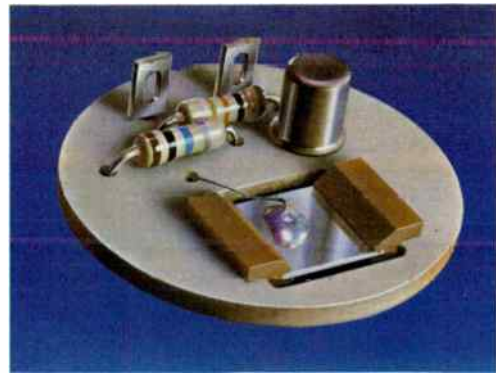
The 'clever bit' of a Philips MFB speaker is this piezoelectric accelerometer (known in the trade as a 'PZE'). This tiny module lives just behind the dust-cap of a MFB speaker's woofer. The ceramic transducer 'chip' is attached to the circuit board with a pair of rubber clamps. Also visible is the FET that, together with the two resistors, forms an impedance converter.
