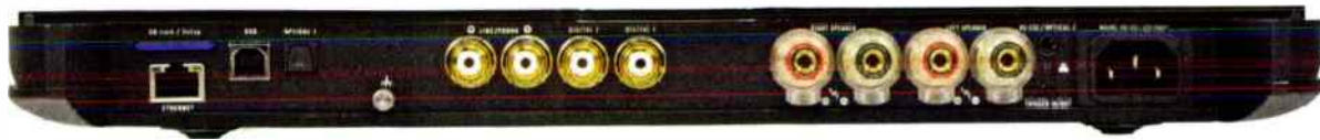
Rear panel connections include digital optical/coaxial, USB and ethernet as well as a configurable line level/phono input - which can accept either MM or MC cartridges.
