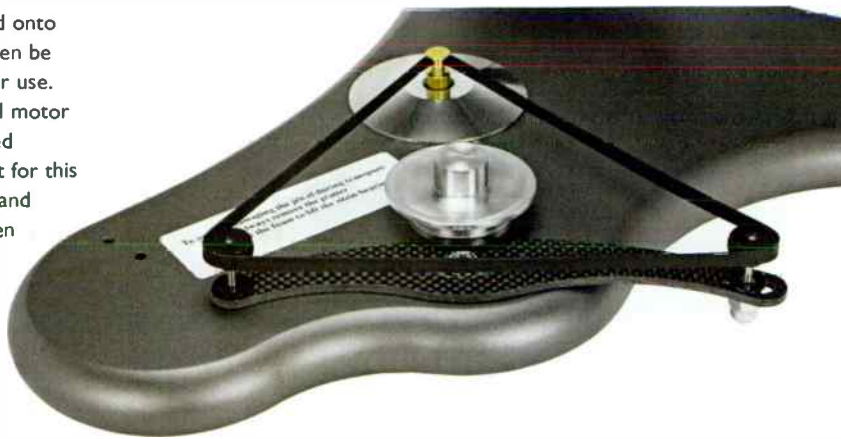
The Vector Drive system with the belt in position to show component disposition. An inner hub underneath the platter engages with the drive belt at three points ensuring an even rotational speed.
