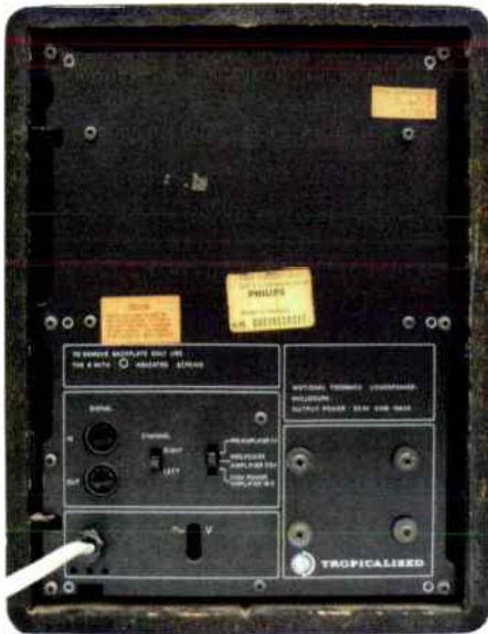
The RH541 is well-connected. The separate input and output DIN sockets, together with the channel switch, ease installation. The three-position sensitivity switch allows the RH541 to be matched to high-level as well as line-level sources.
