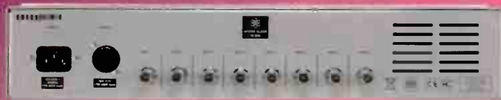
Rear panel of 10M Rubidium clock. It can support eight devices that support 10MHz signal
