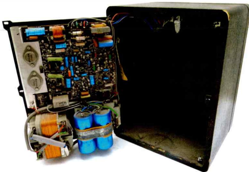
The RH541's electronics were fully discrete and connected to the speaker enclosure by means of a multi-way plug. One of those large blue capacitors (it's 6,800uF) AC-couples the amplifier to the speakers!
