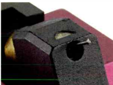
The Ogura PA stylus has dimensions of 3 x 30µm and is attached to a 0.3mm solid boron cantilever.
