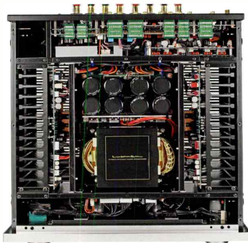
Internally, the Luxman L-590AX MkII demonstrates this company's immaculate build quality and attention to detail. At lower centre is the mains transformer and above it rows of circular smoothing capacitors of the power supply. At left and right are large heatsinks to keep the output transistors cool under Class A operation.
