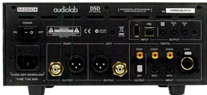
The rear panel carries phono and balanced XLR analogue audio outputs. At right is an XLR socket for balanced (AES/EBU) digital input, alongside electrical and optical digital S/PDIF inputs. There is also a USB B input for computer connection, and USB A for iPhone connection.
