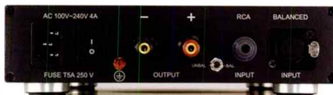
Nu-Force Ref 9V3 SE power amplifier with balanced input, used by Richard Best, behind each loudspeaker.
