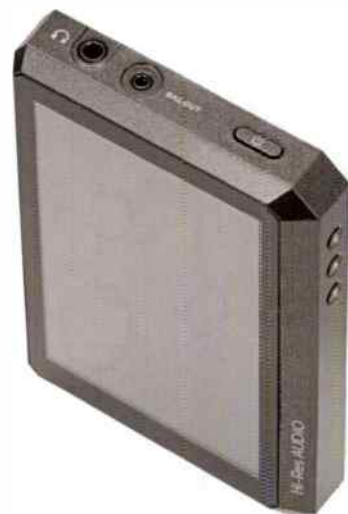
The player's top face carries a conventional 3.5mm stereo headphone jack (left) and a 2.5mm 4-pole balanced output jack.
