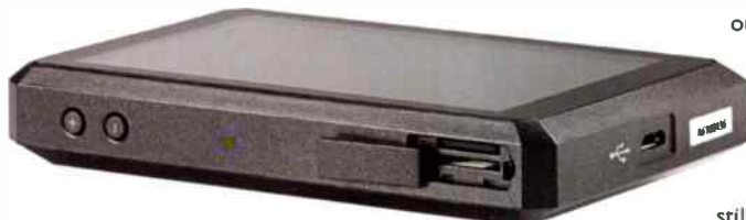
The volume buttons (left) are small. A plastic cover protects its twin microSD card slot.
