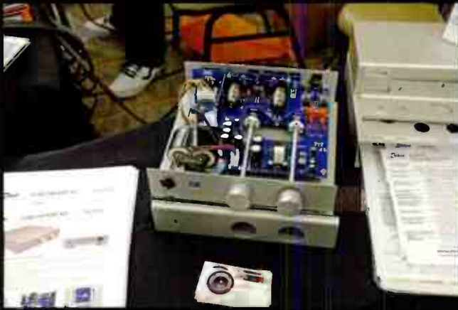
In the foyer I found this very nicely built tube preamp kit, the TU-8500 Elekit from Japan. It uses an R core mains transformer for low hum leakage, plug-in integrated circuits at the front end and ECC82 (12 AU7) output tubes. Go to http://www.elekit.co.jp/en/product/TU-8500 for more details. Price roughly £315.
