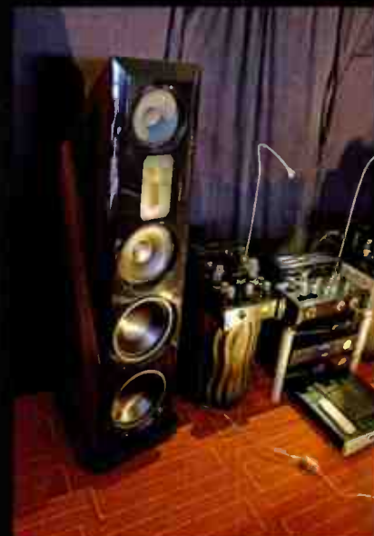
A Legacy Aeris loudspeaker with dual air motion tweeters, open baffle midrange unit, a 10in upper bass unit and two 12in deep-bass units driven by 500W Class D Icepower (B&O) amplifiers. Room correction is provided by an eight-band parametric equaliser. It sounded clear, open and very powerful in a demo.
