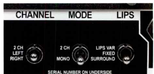
Three switches on the rear of the Elements Power Amplifier allow for a variety of set-up modes, including stereo/monoblock mode.
