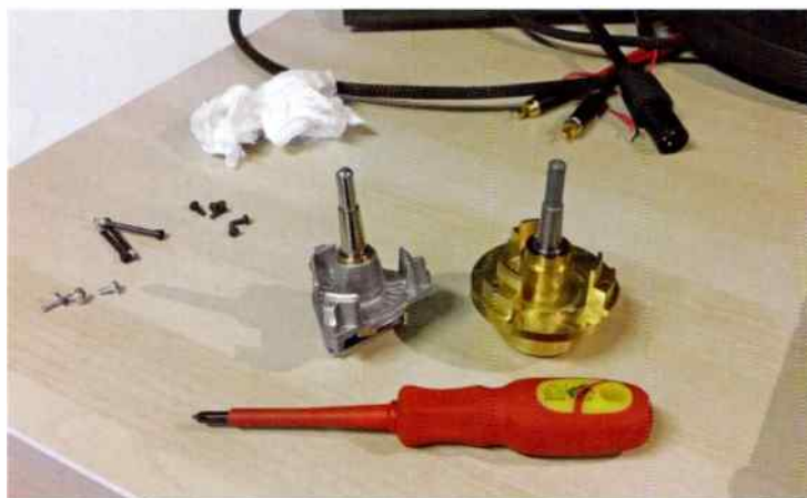
A Mike New brass bodied upgrade bearing for the Technics SL-1210 Mk2. See our February 2015 issue.
