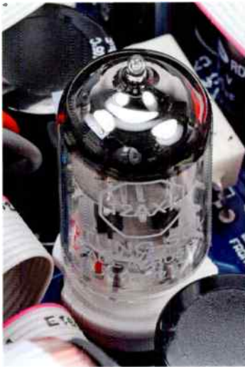
The 12AX7 double-triode driver of the SH is made by Tung-Sol in Russia. 12AX7s are also known as ECC83s.
