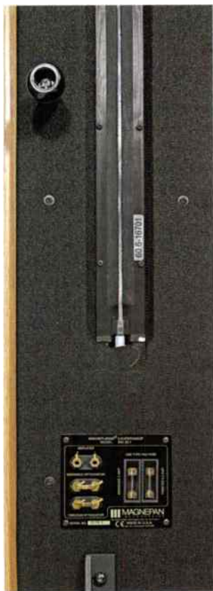
The speaker binding posts sit above the metallic jumpers for tweeter and mid-range tuning. Different resistors are available from Magnepan.
