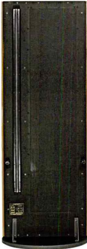
The tall, slim tweeter (high frequency) panel is obvious at rear, firing backwards as well as forwards.
