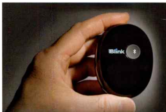
Arcam's Miniblink – a Bluetooth receiver for the hi-fi. Bluetooth uses a unique compression algorithm to reduce data rate of CD and this limits quality, Jon Myles notes.
