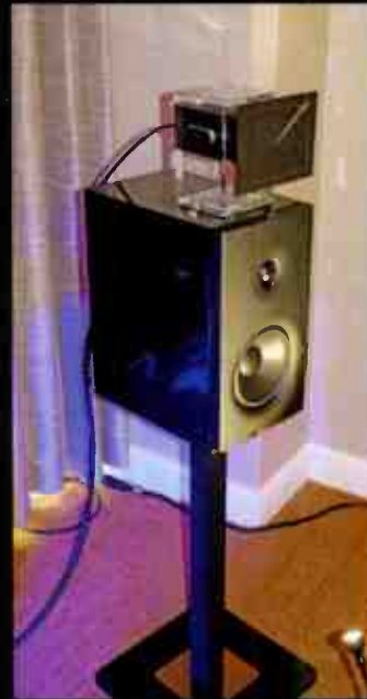
Here's an Enigma self-bias hybrid electrostatic loudspeaker, the Mythology M1. At top is their unique Soprano patented electrostatic super-tweeter that works, I was told, from 8kHz up to 40kHz. Below it lie a conventional fabric dome tweeter and mid/bass unit. See more at www.enigmacoustics.com .
