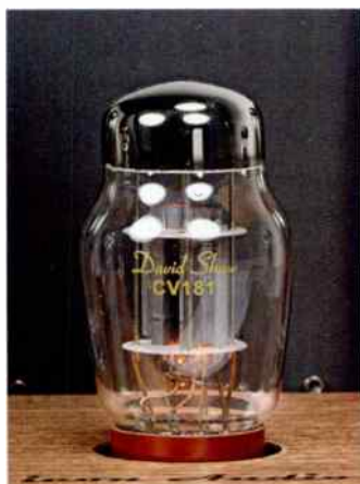
The driver circuit uses three double triode CV181 valves - with Icon Audio's head man David Shaw's name etched on their front.
