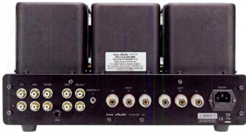
There are 4 Ohm and 8 Ohm loudspeaker taps on the rear (right) as well as CD, Aux and Tuner inputs (left).
