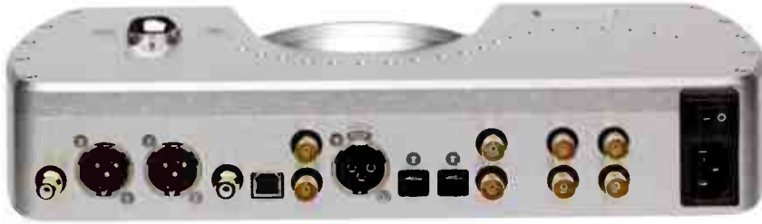
A full set of digital inputs on the rear plus RCA and balanced outputs. Interestingly, on the right there are also four co-axial digital outputs which are said to be for use with forthcoming (but as yet unannounced) Chord products.
