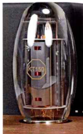
The gherkin-shaped Tung-Sol KT150 Russian-made valve offers exceptional power for a single-ended design.
