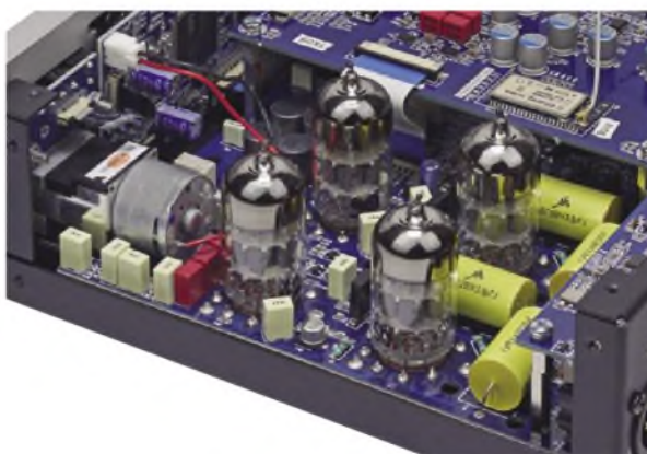
Pre Box RS2 Digital valve stage uses four 6922 twin-triode valves. Motorised Alps volume control at left.
