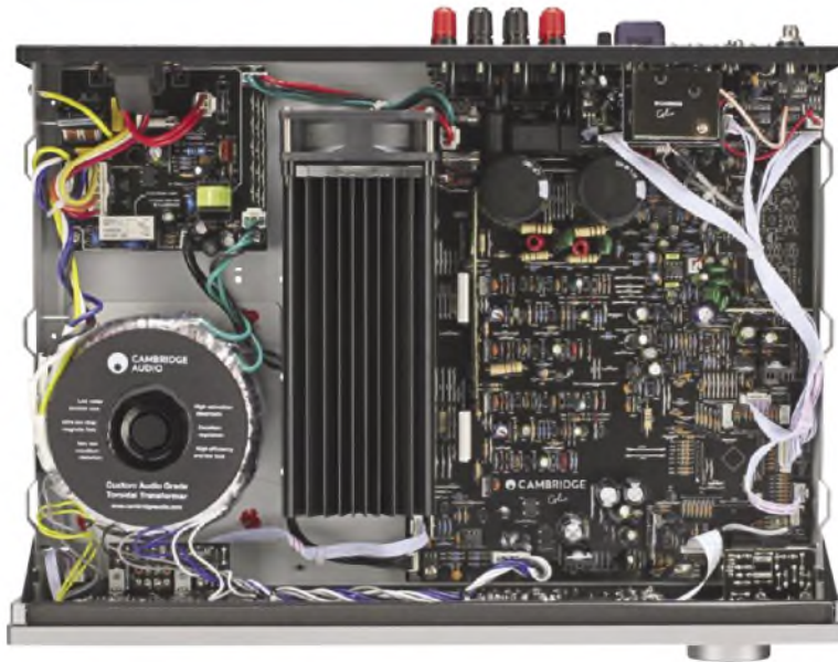
At left is the hefty toroidal mains transformer of the linear power supply and – running vertically down the middle – the heatsink to which the output transistors are bolted. At the top of the heatsink is the somewhat-eager cooling fan that was on the noisy side. Digital sources, including the Bluetooth receiver and Colin’s SDR module, are mounted on the rear panel.
