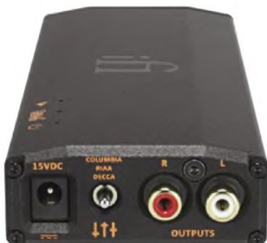
The 'front' of the case – or is it the back? Outputs and a small three-way toggle switch to select standard RIAA, Decca or Columbia playback EQs.
