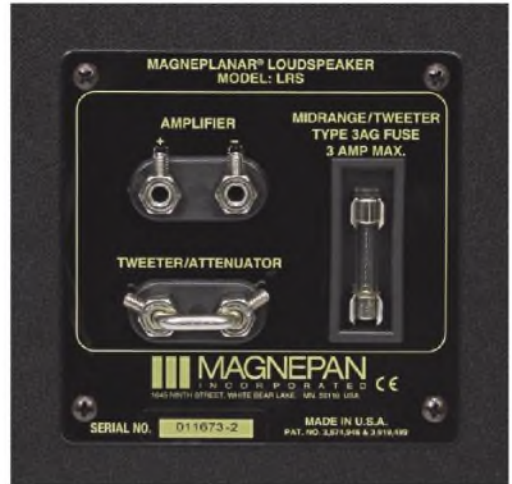
The unusual connecting panel of the LRS. It accepts 4mm plugs or bare wires of 4mm diameter, secured by a hex-key grub screw. The Tweeter/Attenuator link can be replaced by a resistor to reduce treble.
