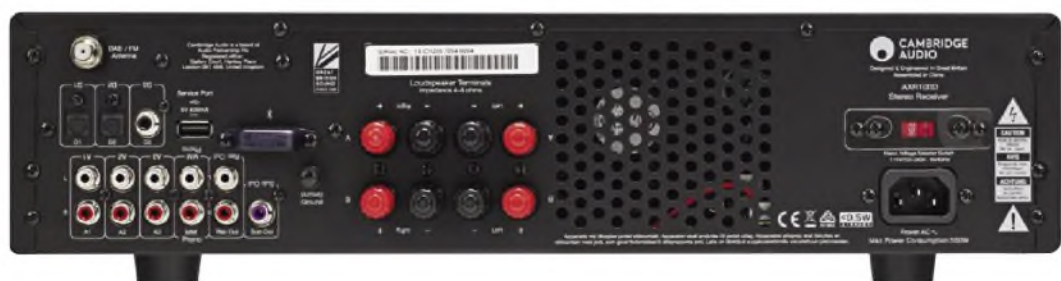
Plenty of connectivity here – three line-level analogue sources, plus MM phono. There's a mono subwoofer and recording output, but no tape loop. A single aerial socket is used for both VHF/FM and DAB. Four external digital sources – two optical, one coaxial and Bluetooth – are catered for. Bluetooth is built in, not reliant on a USB dongle (there is a USB port, but it's for service purposes). For the output, Cambridge has specified decent terminals – bare wire or banana plugs – for two pairs of speakers.
