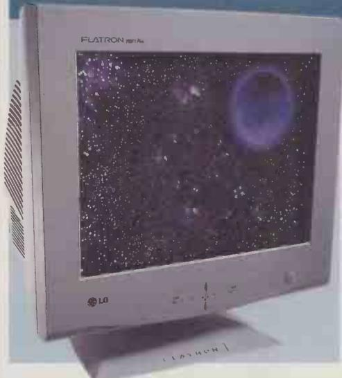
**CONVENTIONAL CRTS** are still based on a screen that is formed from part of a glass sphere – or a cylinder for Sony's Trinitron displays. However, some screens are designed with a completely flat front surface such as Mitsubishi's Diamondtron NF and FD Trinitrons. Although these tubes can produce wonderful results, the internal surface remains curved to compensate for beam diffraction. This is where the LG Flatron differs as both sides of its tube are flat.
