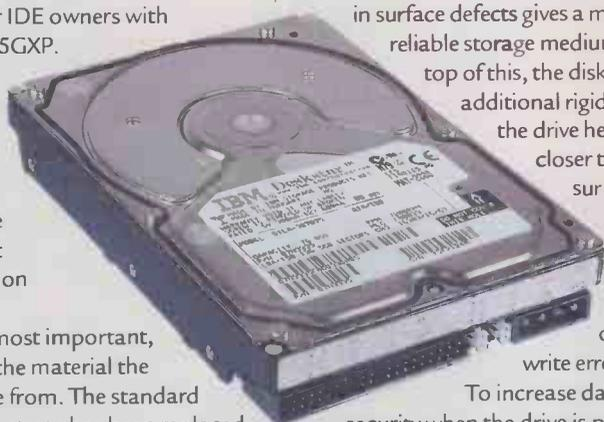
The glass substrate also undergoes a manufacturing process to create a smoother disk. The subsequent reduction in surface defects gives a more reliable storage medium. On top of this, the disk's additional rigidity allows the drive heads to fly closer to the surface, cutting down the number of read/write errors.
