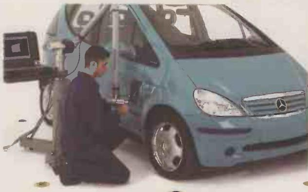
3D scanner in action mapping a Merc A Class
