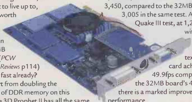
larger heatsink between them. There is also a second PCB riser above the first to deal with the S-Video electronics as well as a DVI output.
